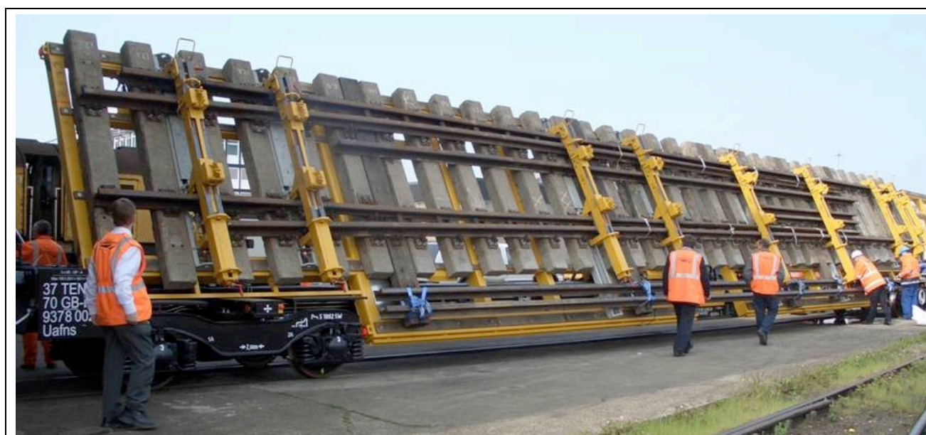
Figure 3 Transport of pre-assembled S&C panel – Network Rail modular S&C initiative 4
