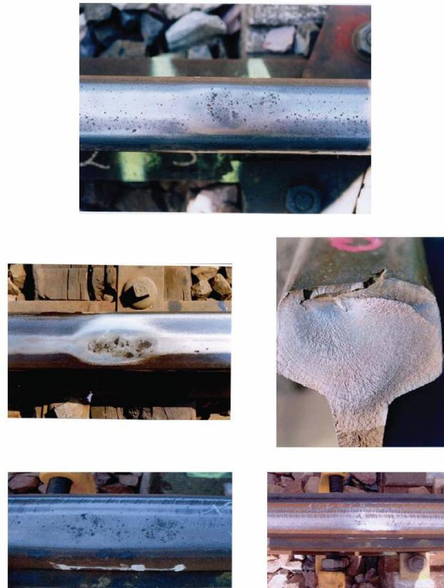
**Figure 5 - Photos of Squats. Examples of surface appearance (dark spot) and transverse crack development**
