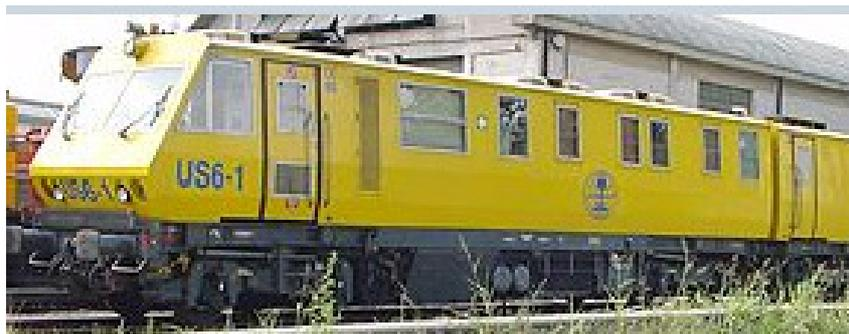
**Figure 35 - Speno US 6-1 Ultrasonic Rail Testing Vehicle.**
