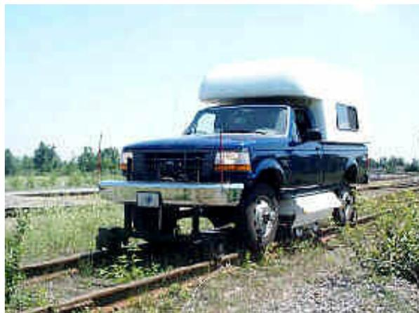
**Figure 7 - EMAT inspection system for automated rail inspection mounted on a hi-rail vehicle (Tektrend).**
