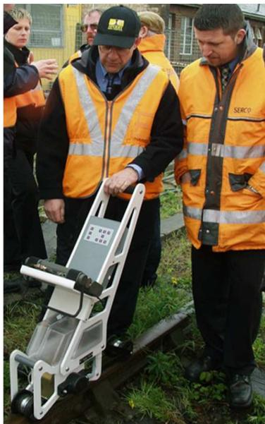
**Figure 9 - Portable ultrasonic rail inspection unit (Sperry stick)<sup>4-5</sup>.**
