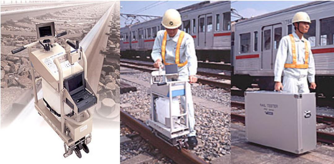
**Figure 29 - Tokimec Ultrasonic Rail Flaw Detector**
