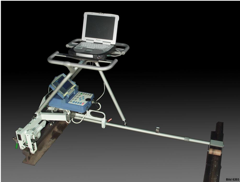
**Figure 15 - Manual inspection of rails with eddy current sensors (photo courtesy of DB).**
