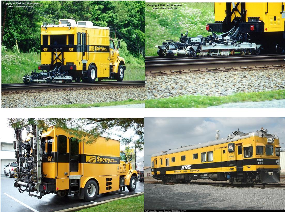
**Figure 25 - Sperry rail services ultrasonic testing cars and railway vehicles.**
