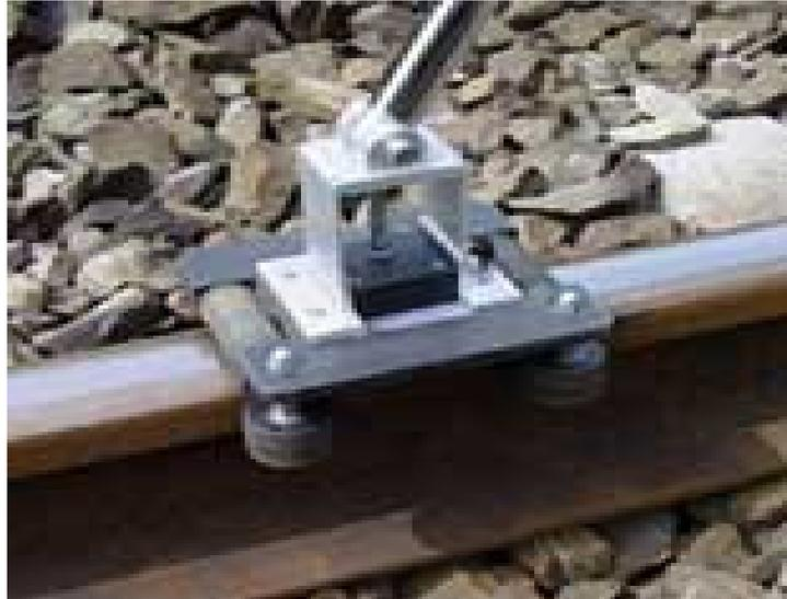
**Figure 14 - EC sensor for detection of RCF cracks on rails (Hocking NDT).**
