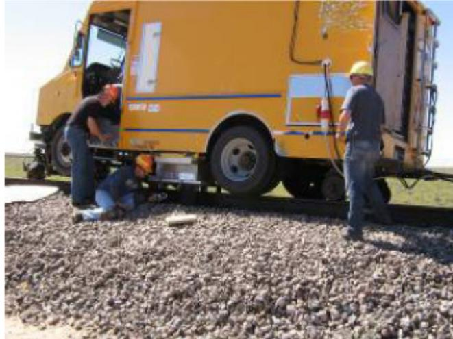
**Figure 21 - The TTCI-Technogamma laser ultrasonics hi-rail vehicle<sup>13</sup>.**
