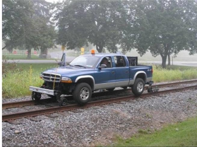
**Figure 8 - Photograph of a hi-rail vehicle incorporating a long-range ultrasonics system for the inspection of transverse cracks.**
