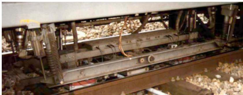
**Figure 33 - Ultrasonic probes mounting**
