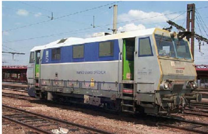
**Figure 32 - SNCF ultrasonic inspection train**
