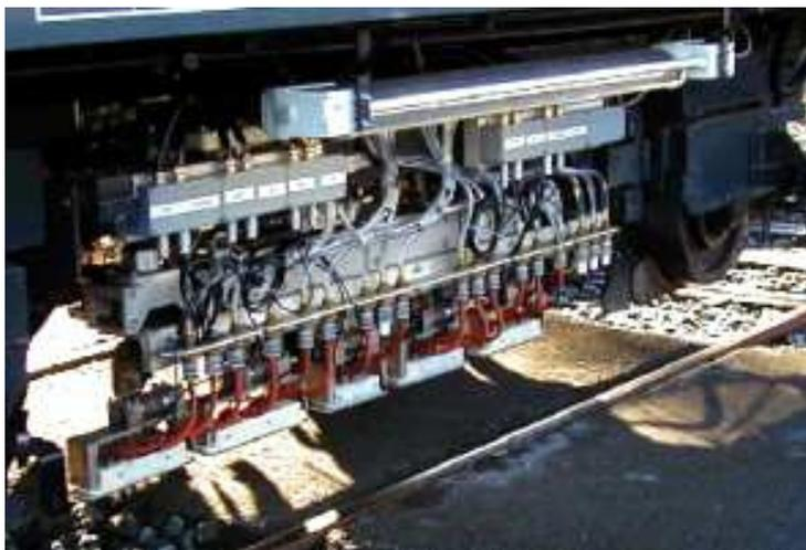
**Figure 10 - A five-sled arrangement shown lifted off the rail. Some of the sleds include two probes which allow a total of seven ultrasonic probes to be used. A four-sensor eddy current probe (not shown) can be similarly mounted<sup>29</sup>.**
