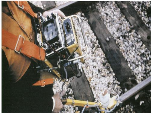
**Figure 23 - Ultrasonic Rail Flaw Detection (URFD) equipment.**
