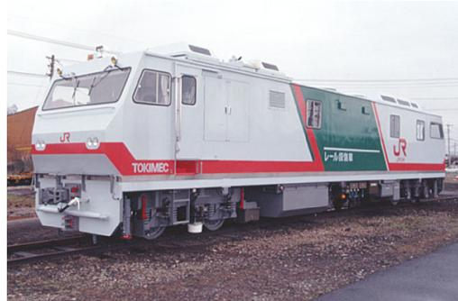
**Figure 28 - Tokimec Ultrasonic Rail Inspection Car 'URIC'**
