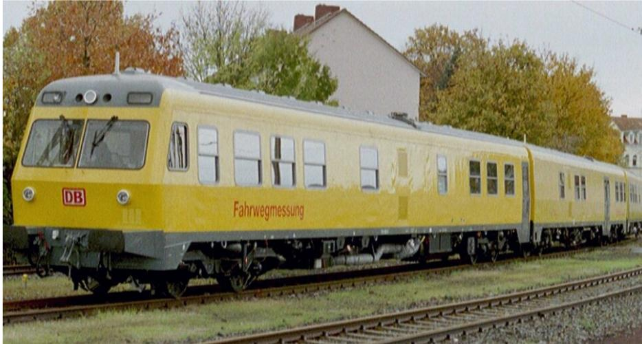
**Figure 26 - EURLSCOUT UST 02 Eddy Current and Ultrasonic Measuring Train (courtesy of DB)**
