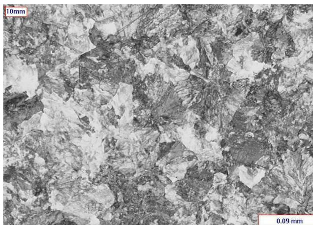
**Figure 2** *Optical microscope image, rail disc INR10, material VA 350 grade, 10mm under the surface. Test INNOT-04, 5000 cycles dry.*
