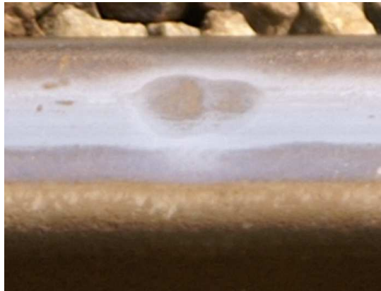
Figure 9 A squat developed from a wheel burn
