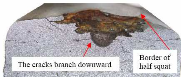
(b) Cross-section of the broken rail at the squat
