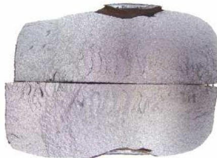
(b) The cross-section of the broken squat
