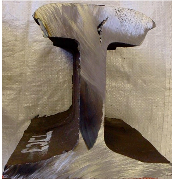
Figure 9: gross plastic deformation of a low rail in highly canted curve
