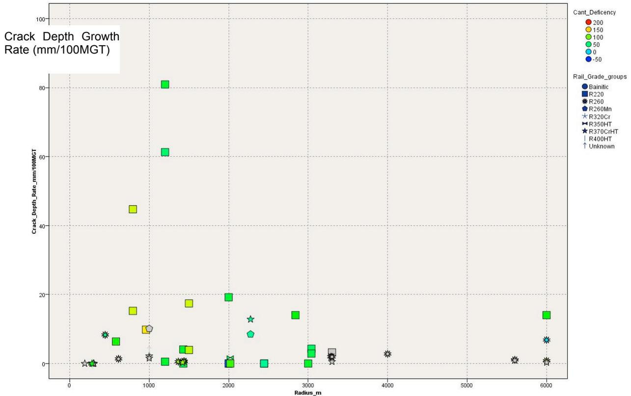
Figure 13: Crack depth growth rate
