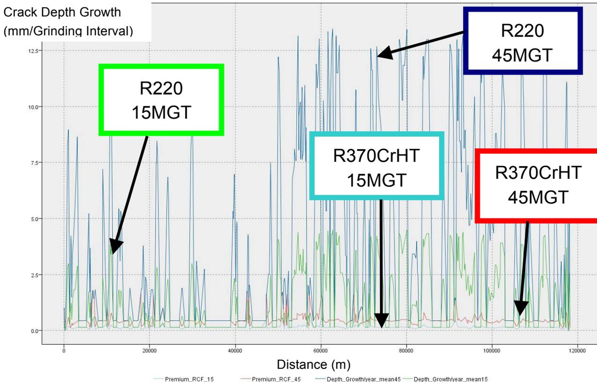
Figure 31: Effect of grinding interval on depth of RCF crack, premium grades applied to curves of <2700m
