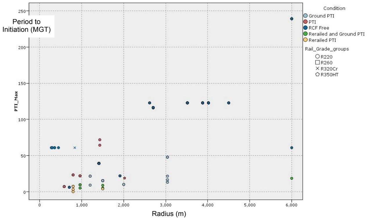
Figure 23: Period to initiation of RCF cracks
