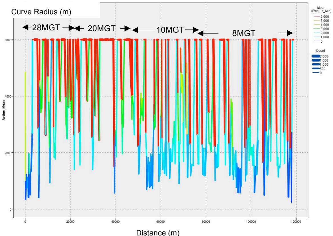
Figure 24: Radius profile of route (tangent track drawn at a radius of 6000m)
