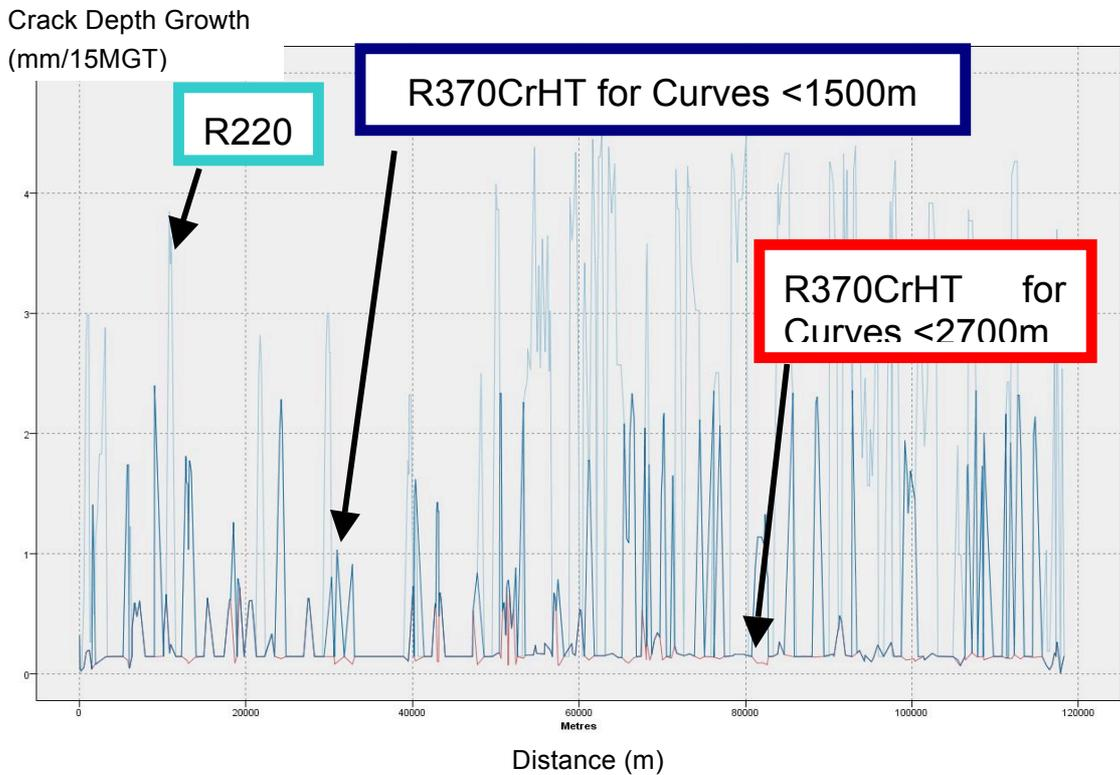
Figure 29: Premium Grade Rails and RCF crack depth growth per 15MGT
