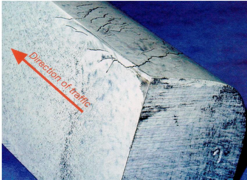
Figure 21: RCF crack growth[25]
