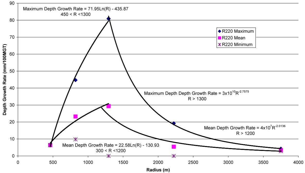
Figure 16: Crack depth growth rate for grade R220
