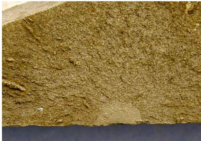
*Figure 3: Rail breakage from a fatigue crack initiating at a corrosion pit*
