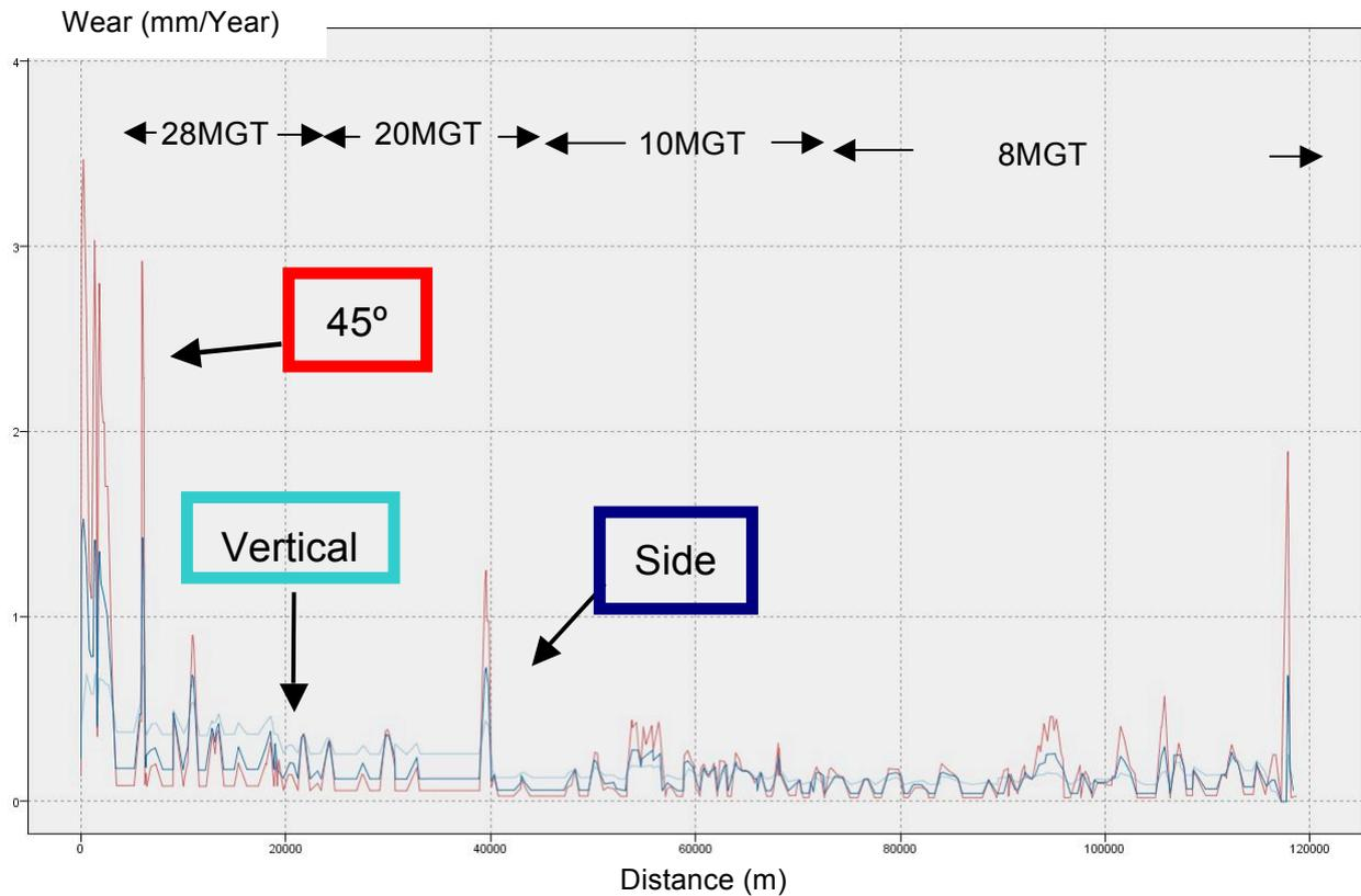
Figure 26: Comparison of predicted wear for full route (based on R220)
