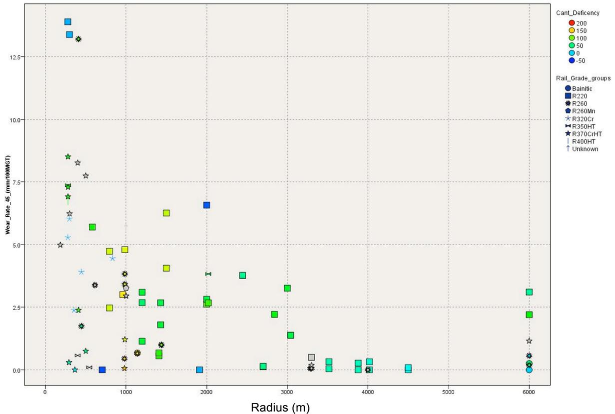
Figure 8: 45° Wear rate for different rail grades
