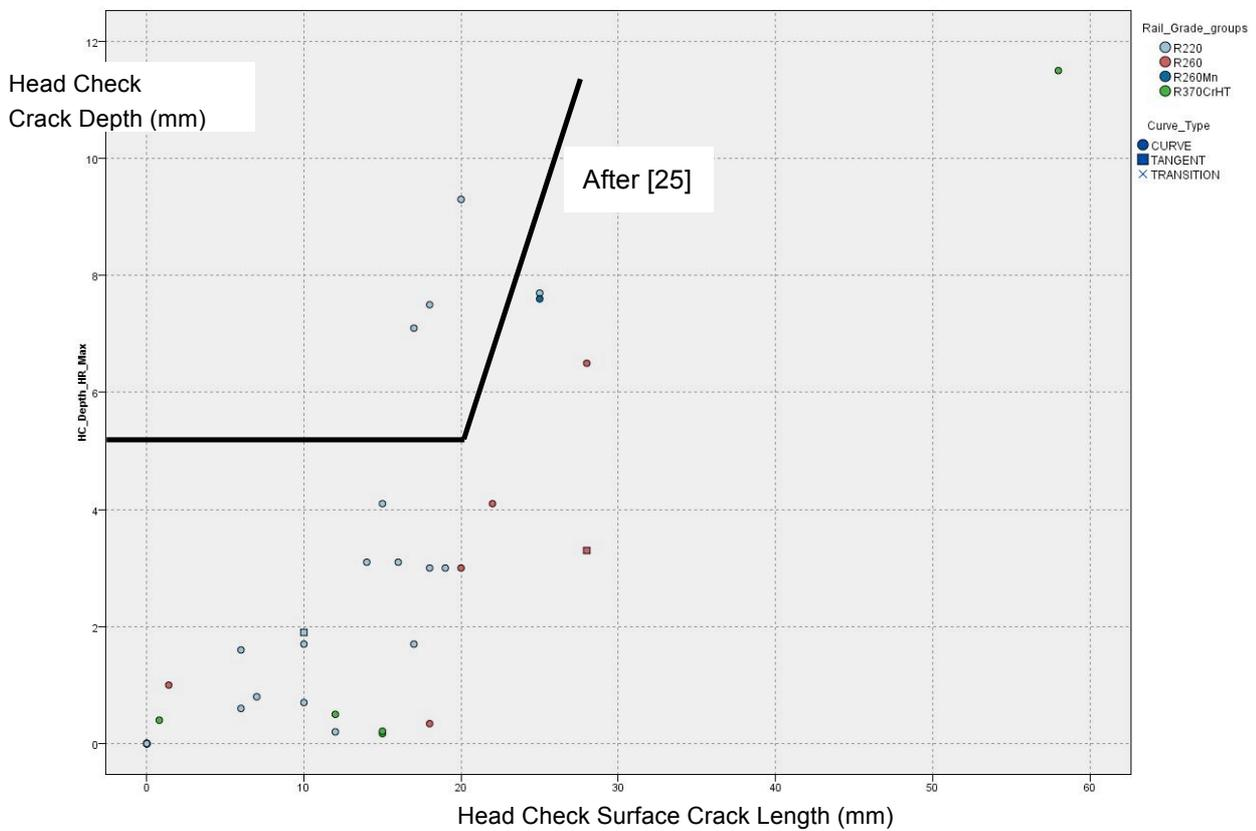
Figure 20: Crack depth against surface crack length
