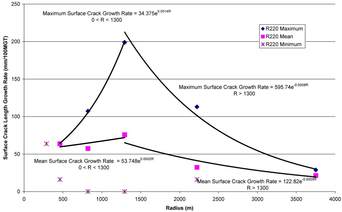
Figure 17: Surface crack growth rates for grade R220
