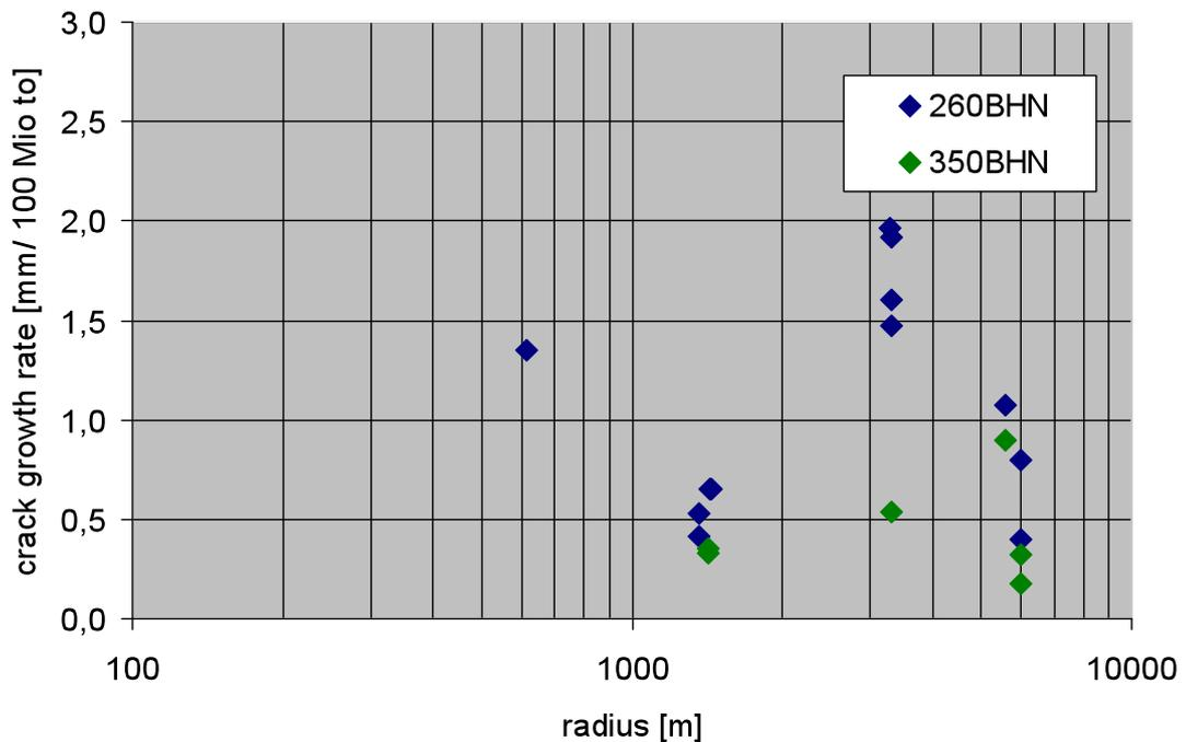
Figure 15: Comparison of RCF crack growth of grade R260 and R350HT
