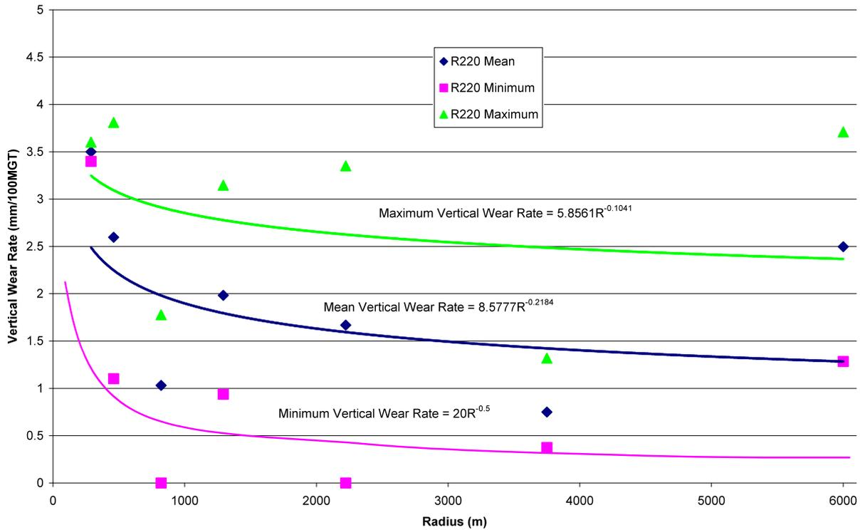
Figure 9: Vertical Wear Rate of Grade R220
