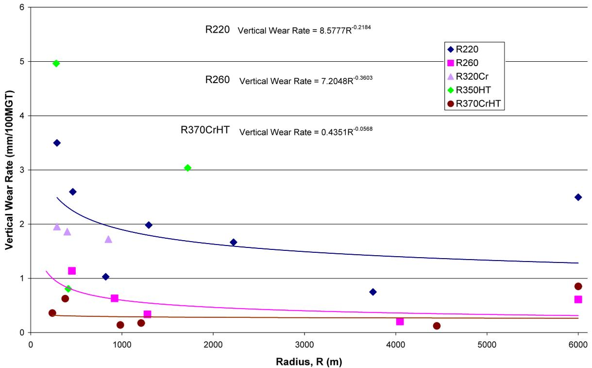
Figure 11: Mean vertical wear rate for all rail grades
