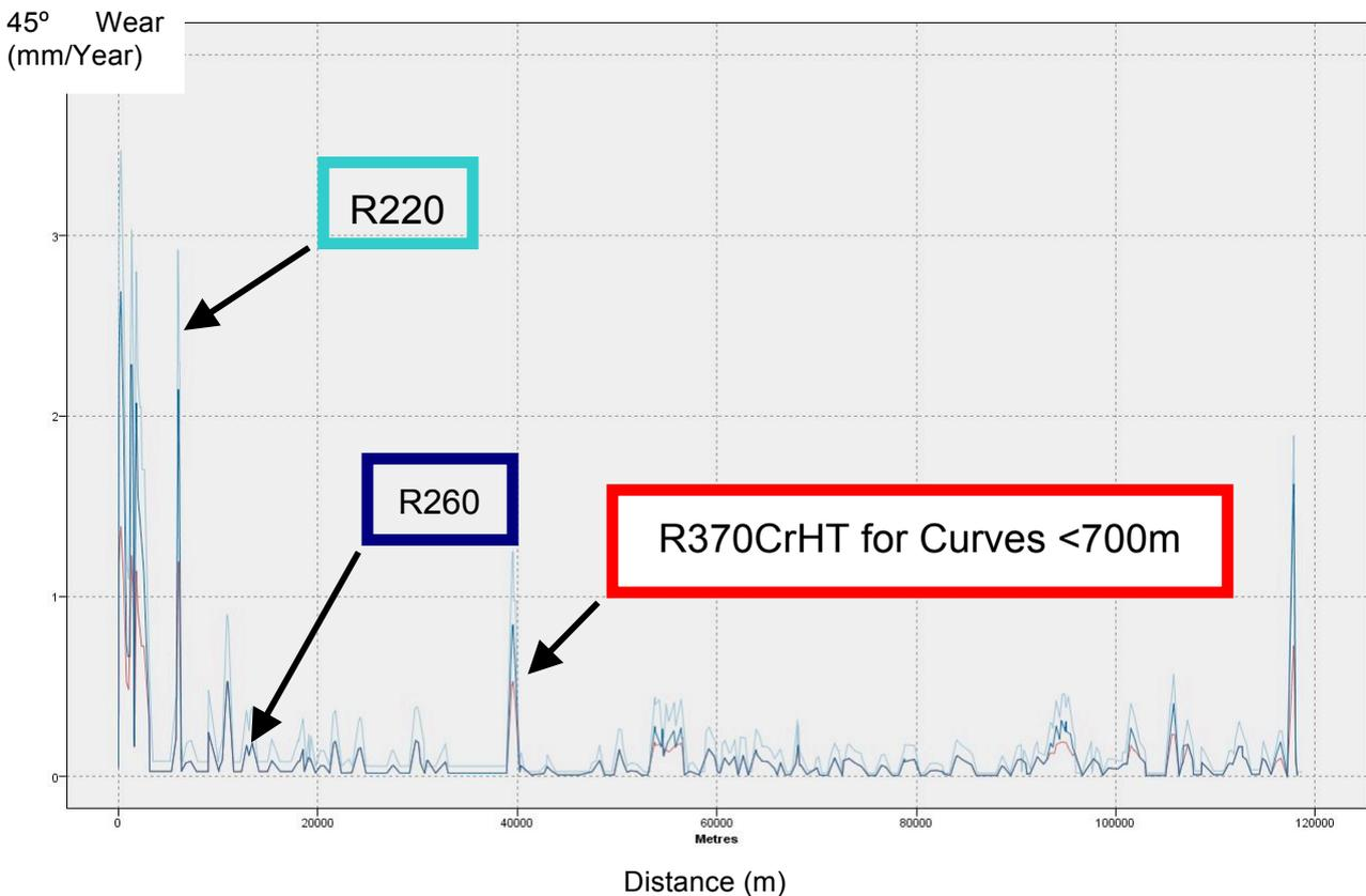
Figure 27: Effect of Premium Grade Rail Steels on Wear
