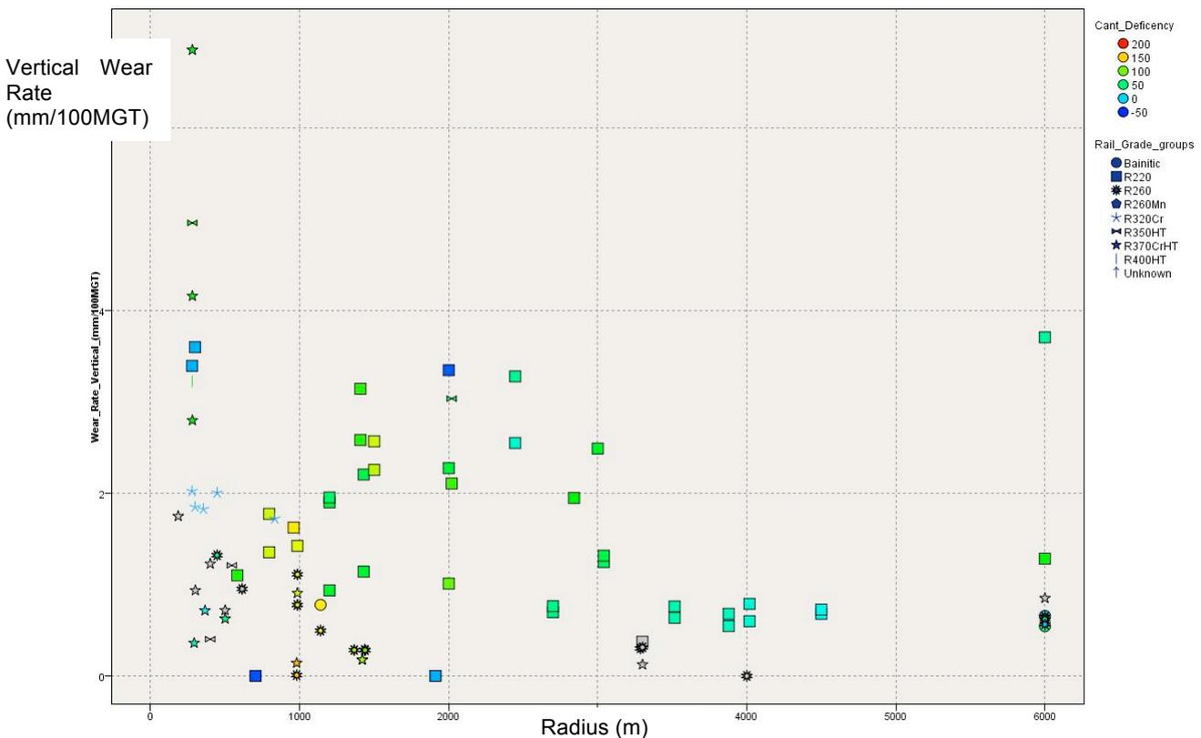
Figure 7: Vertical wear rate against radius for different rail grades
