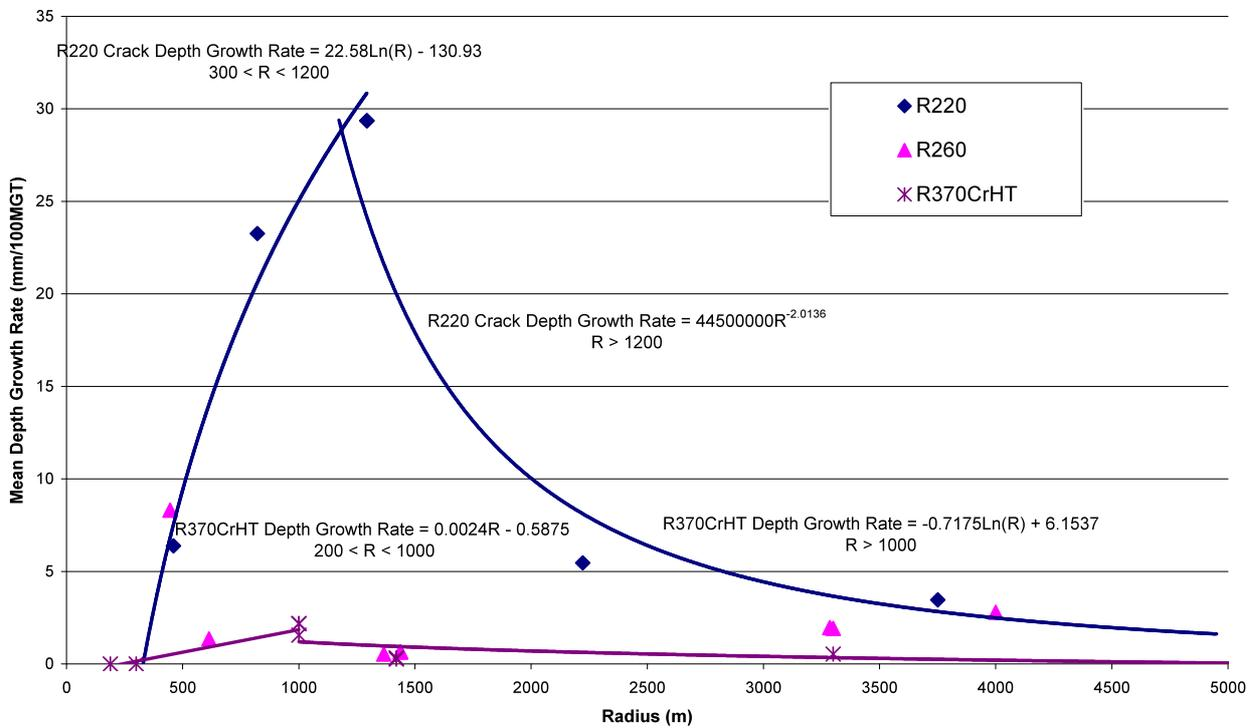
Figure 18: Mean crack depth growth rates for all rail grades
