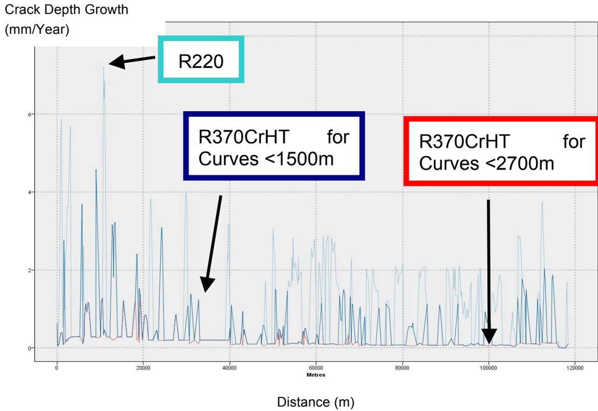
Figure 28: Premium Grade Rails and RCF crack depth growth per year
