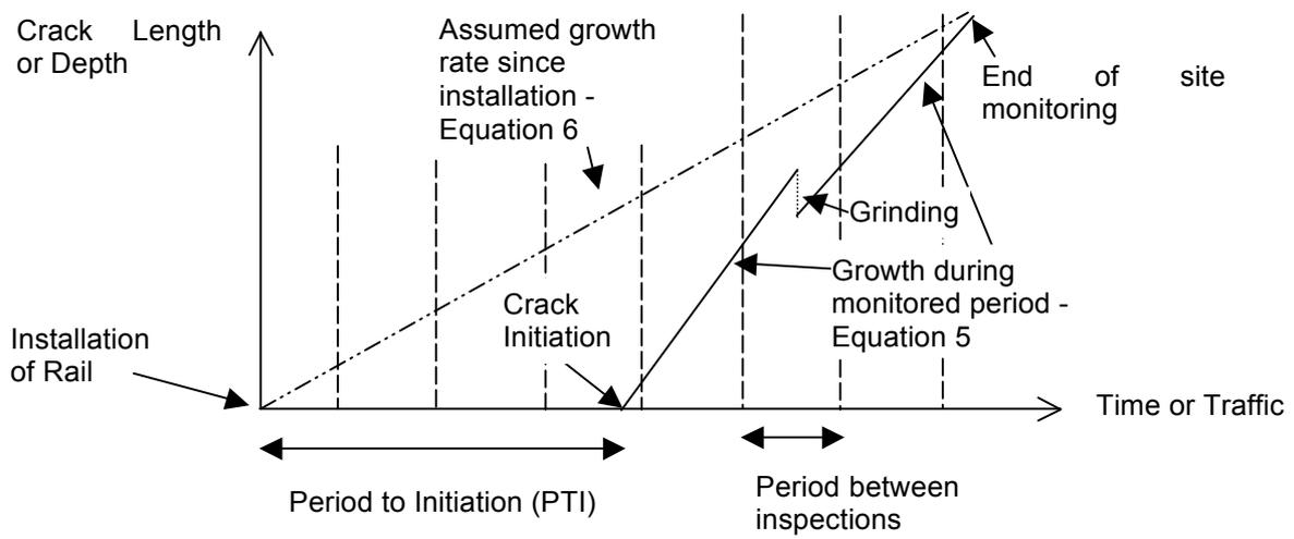
Figure 6: Schematic of inspection cycle superimposed on RCF crack development
