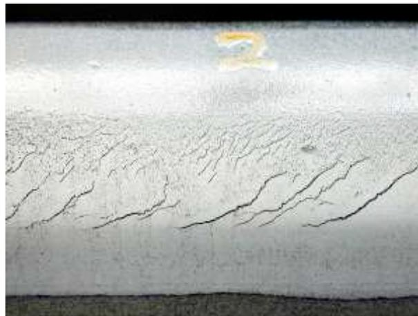
*Figure 2: RCF Cracks (head checks)*
