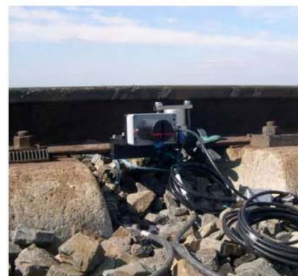
Fig. 27: Cross sections where track stiffness was measured
