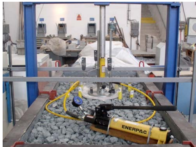
Fig. 14: Static plate load test
