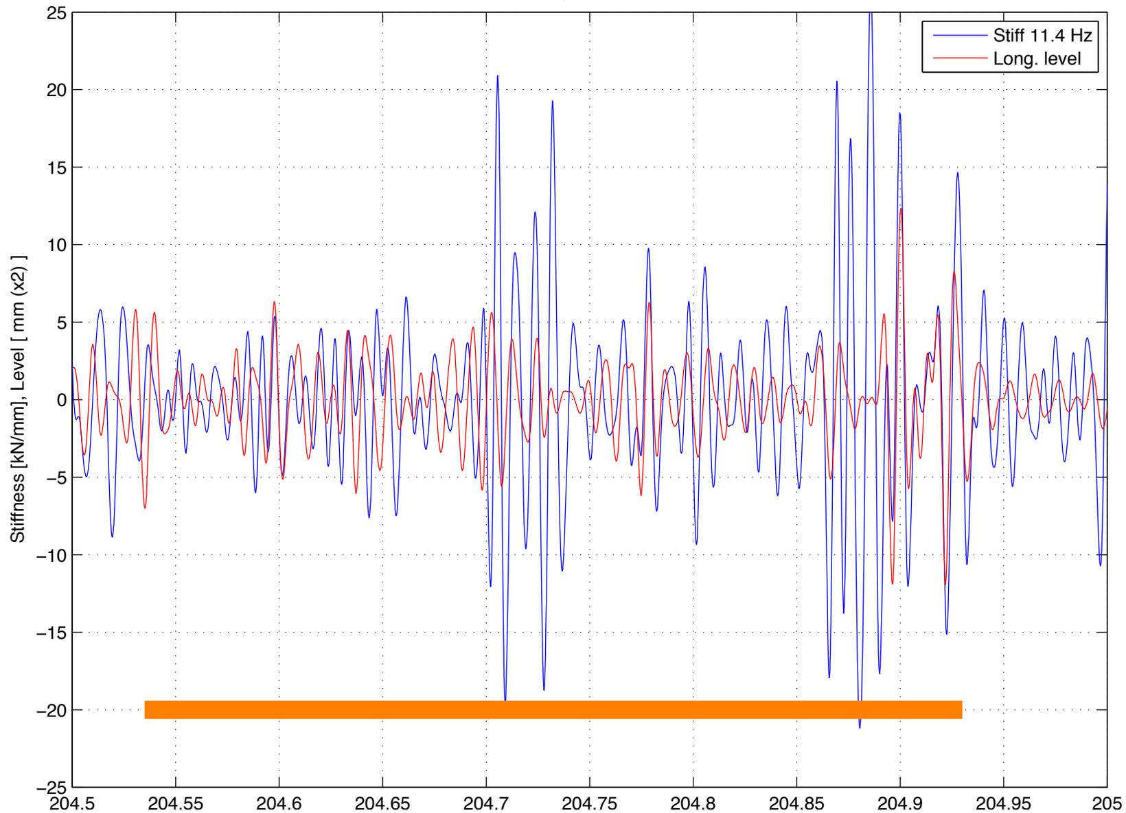
RSMV measurement 40 km/h, stiffness and long. level  $\lambda = 5-15$  m Czech republic, Section 3, track 1
