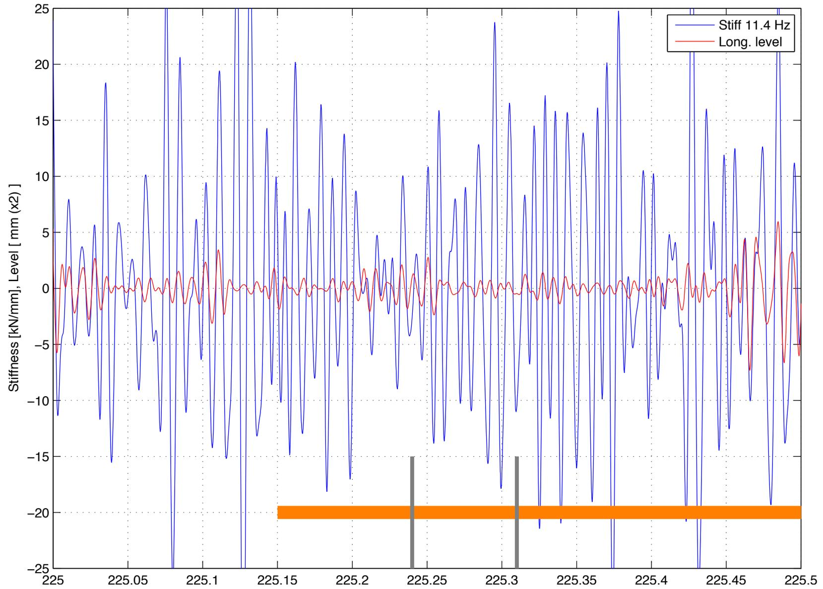
RSMV measurement 40 km/h, stiffness and long. level  $\lambda = 5-15$  m Czech republic, Section 3, track 2
