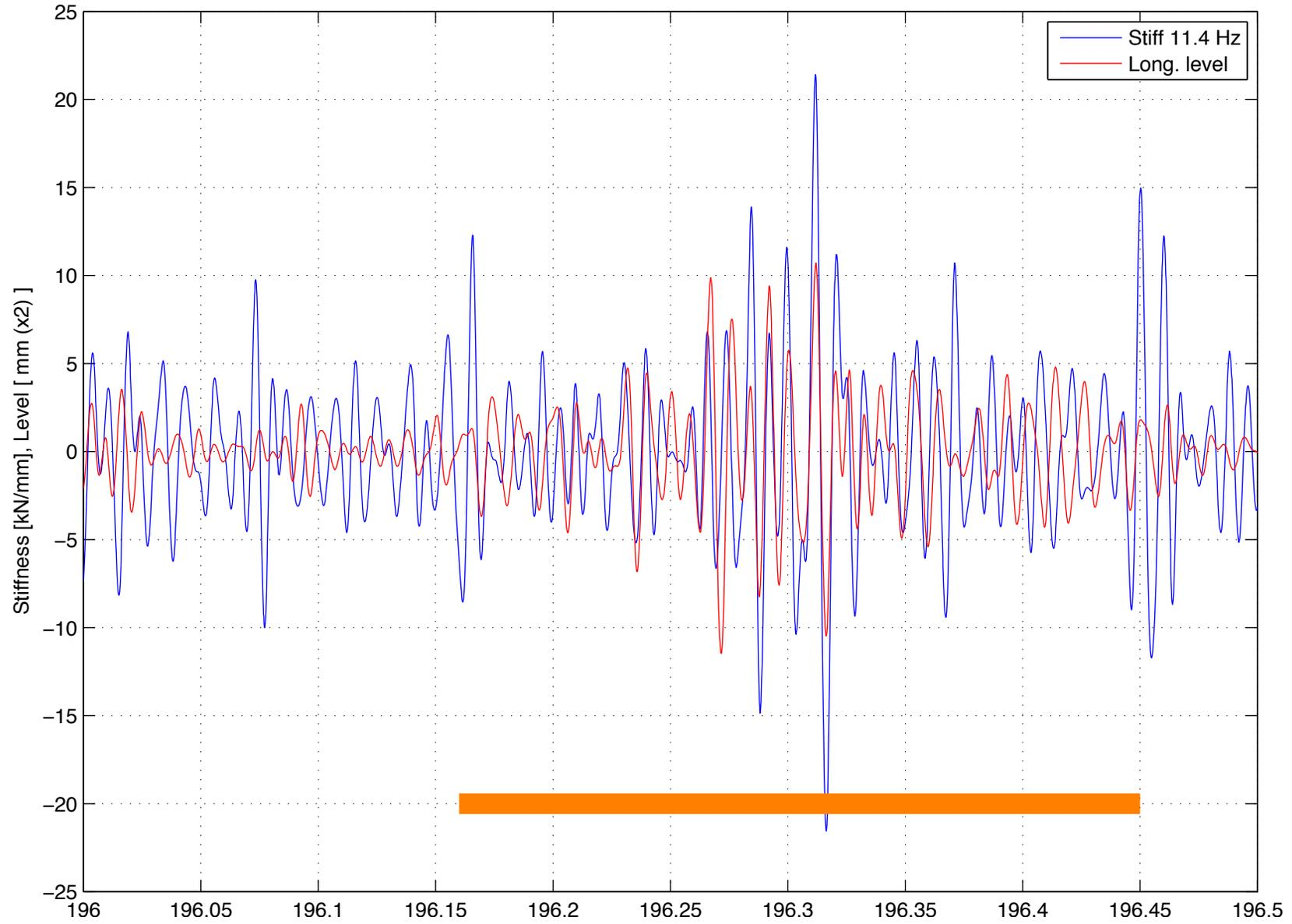
RSMV measurement 40 km/h, stiffness and long. level  $\lambda = 5-15$  m Czech republic, Section 1, track 1
