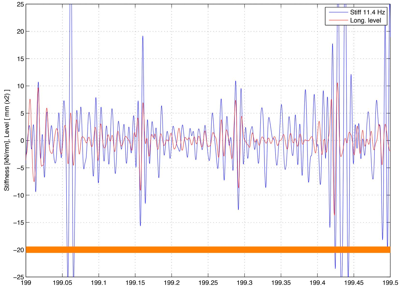
RSMV measurement 40 km/h, stiffness and long. level  $\lambda = 5-15$  m Czech republic, Section 2, track 2
