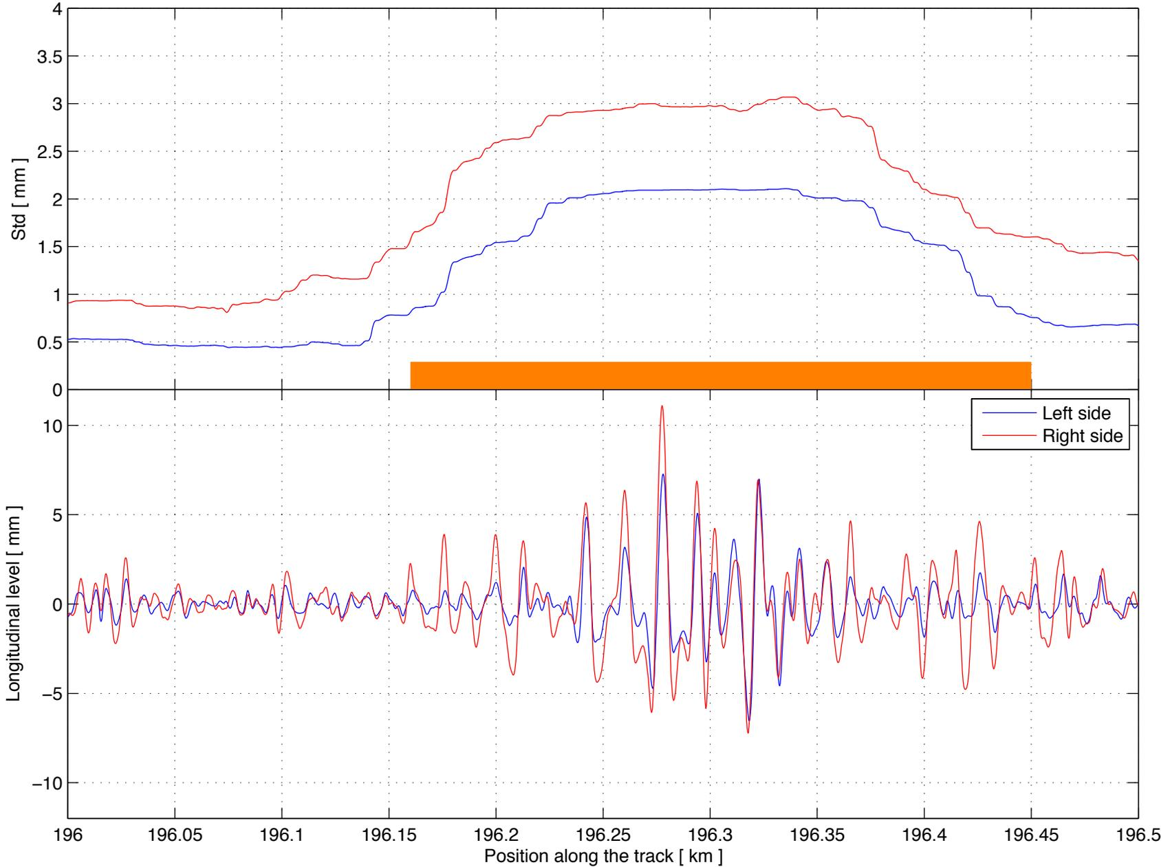
RSMV measurement 40 km/h, no excitation (longitudinal level) Czech republic, Section 1, track 1
