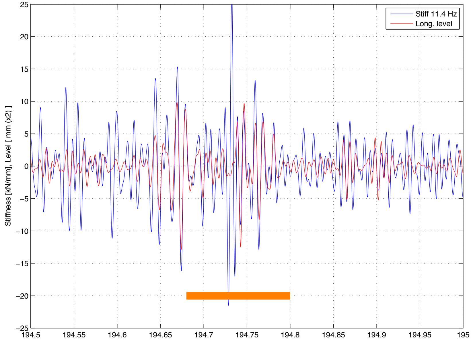
RSMV measurement 40 km/h, stiffness and long. level  $\lambda = 5-15$  m Czech republic, Section 1, track 2
