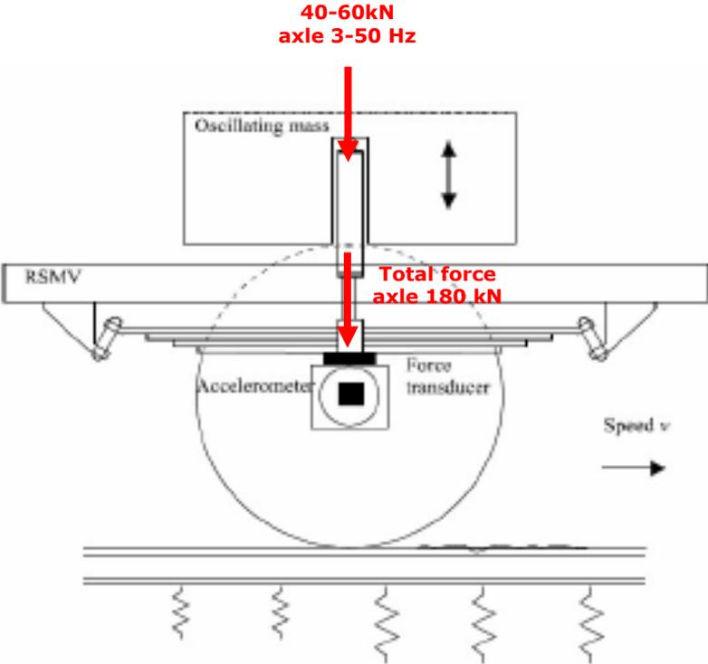
Figure 3.1 RSMV measurement principal and force transfer
