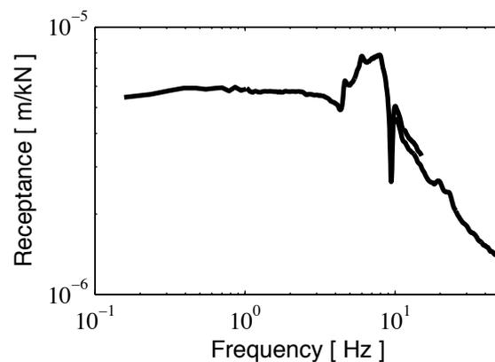
Figure 3.3: a: Vertical force-deflection diagram of track with quasi-static excitation (measured on rail), b: Magnitude of vertical track receptance with subsoil of clay (measured on rail),  $F_{\text{stat}} = 90 \text{ kN}$ ,  $F_{\text{dyn}} = 10 \text{ kN}$ . Measurements made by Banverket with standstill track-loading test vehicle in Sweden.
