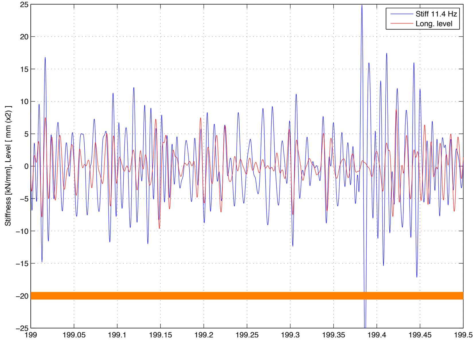
RSMV measurement 40 km/h, stiffness and long. level  $\lambda = 5-15$  m Czech republic, Section 2, track 1
