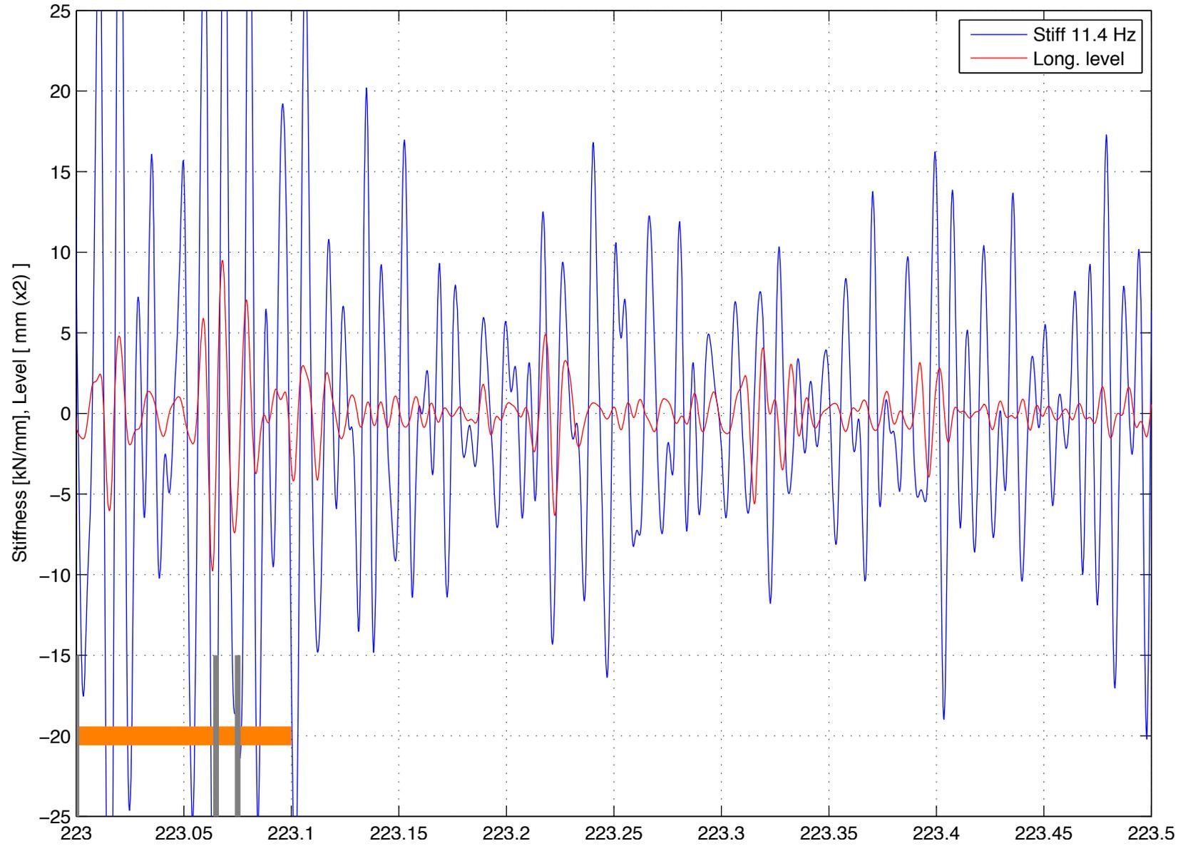
RSMV measurement 40 km/h, stiffness and long. level  $\lambda = 5-15$  m Czech republic, Section 3, track 1
