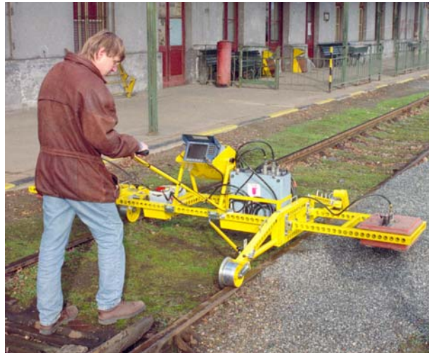
Fig. 1: GPR apparatus with antenna systems on rail trolley CRAB. The same apparatus can be installed in track recording car or on engine front.
