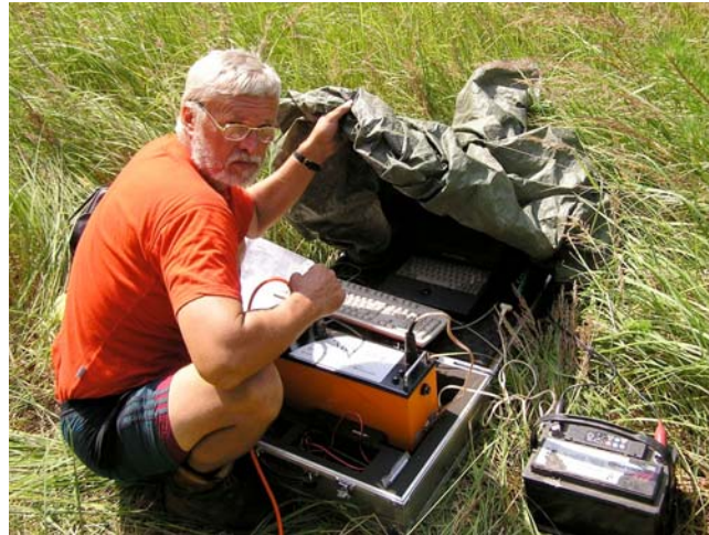
Fig. 2: Apparatus controlling a multielectrode system during fieldwork.
