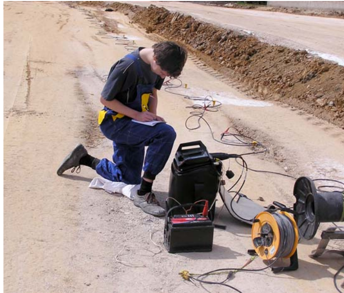
Fig. 3: Seismic apparatus during the measurement in the field.
