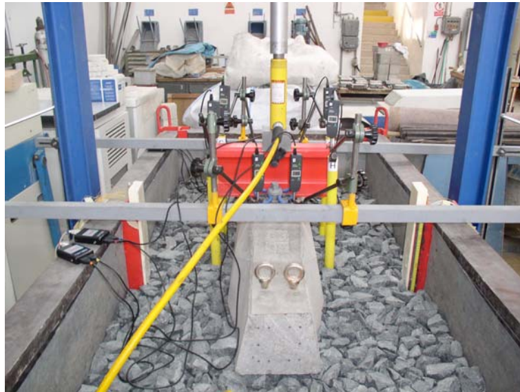
Fig. 3 Measurement of settlement under short-term loading
