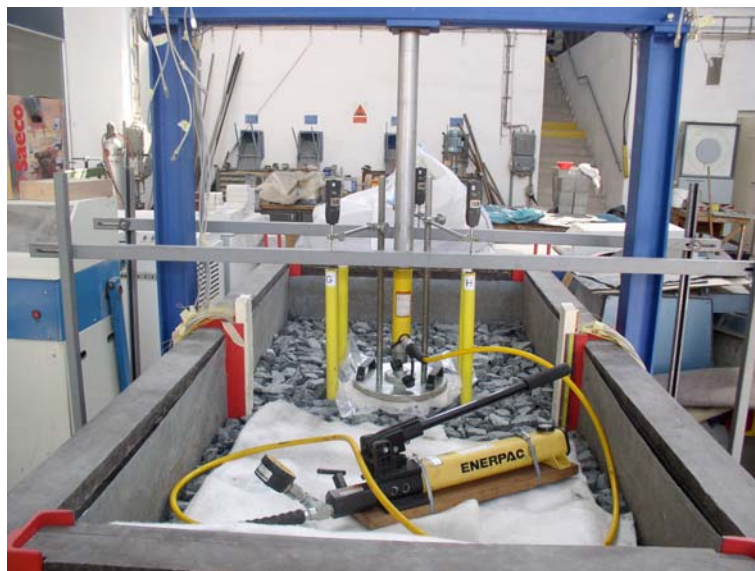
Fig. 4 Static plate load test
