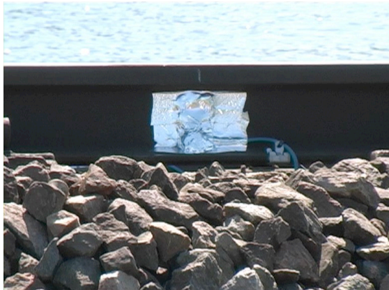
Figure 5.3: Several strain gauges are mounted in a specific pattern on both rail webs. They are all fully encapsulated.
