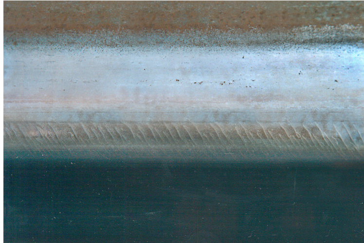
Figure 5: Head Check of category 3; source DB regulation 821.2007A02
