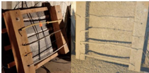
As the fibre optic sensor is still sensitive to knocks and handling, any section of fibre installed must be mechanically protected, it must not remain exposed to air. The sections of measurement length
