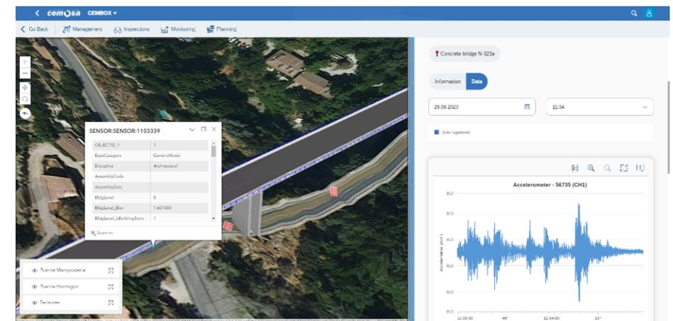
Figure 58-2. CEMBOX Infra Monitoring interface.
