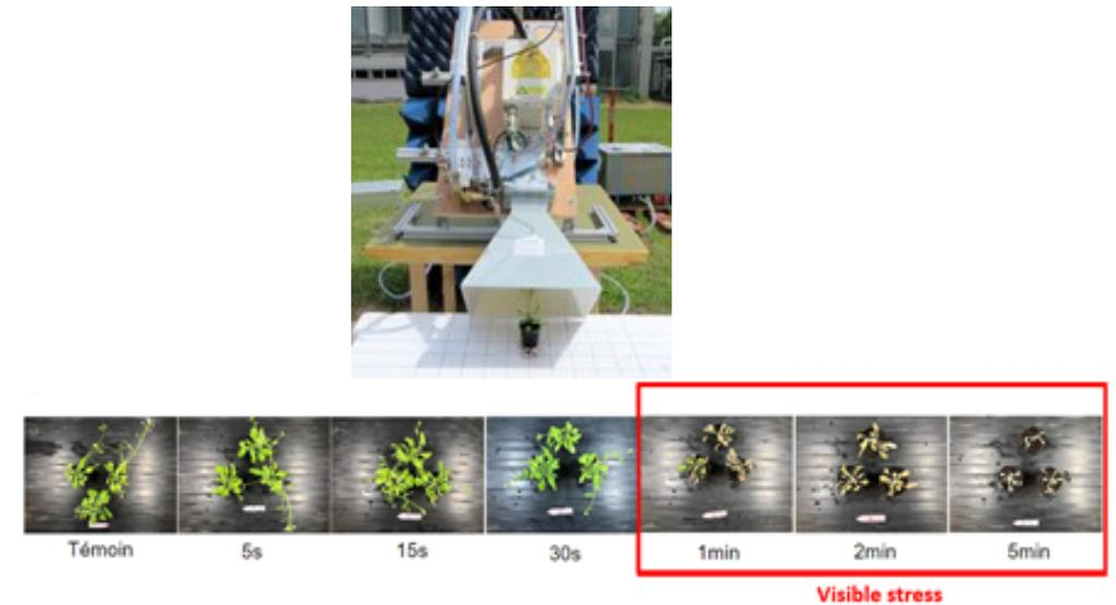
Figure 32-2 Thermic exposition study setup and example of results
