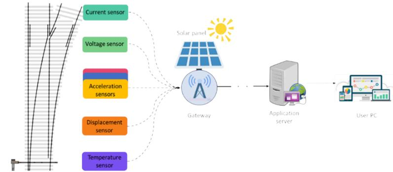
Figure 1-1 Overall scheme of a sensor network
