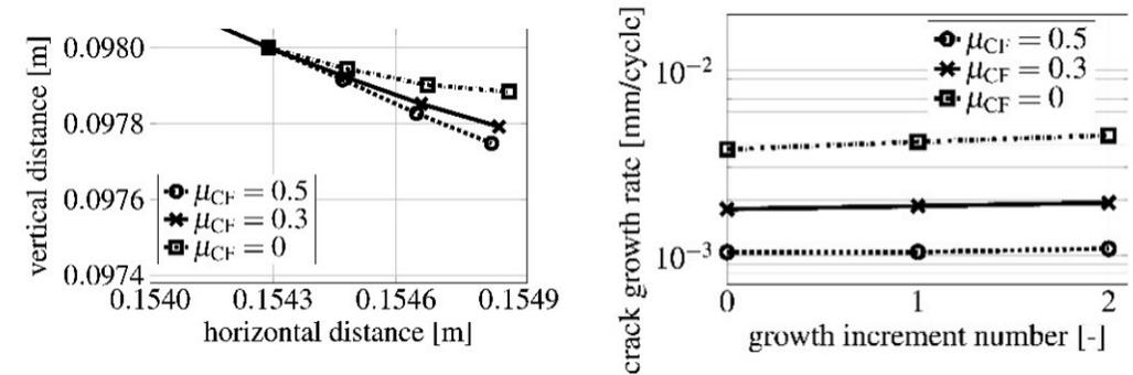
Figure 48-1 (top) A 3D rail model with a gauge corner crack. (bottom left) Zoom-in of predicted 2D crack paths for different levels of crack face friction ( $\mu_{CF}$ ) under pure contact load. (bottom right) Predicted 2D crack growth rates for different levels of crack face friction ( $\mu_{CF}$ ) under pure contact load
