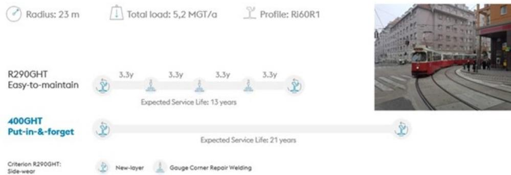
Figure 64-1 Life Cycle prognosis based on linear wear models.
