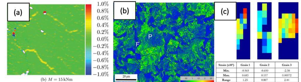
Figure 27-1 (a) Cracks on rail surface identified with DIC [1]. (b) Local misorientations in wheel steel ER7T after heat treatment (ht) at 500 °C; ferrite grains (blueish) have smaller gradients than the pearlite [2]. (c) Residual strains in ferrite grains (ER7T after ht at 500 °C) measured by synchrotron X-ray diffraction [3].
