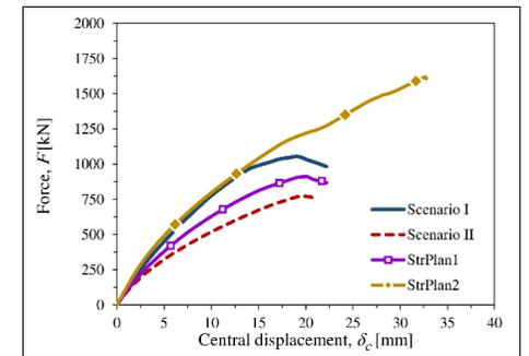
Figure 56-3 Load-deflection of undamaged (Scenario I) and damaged (Scenario II) RT, and after strengthened according to StrPlan1 and StrPlan2
