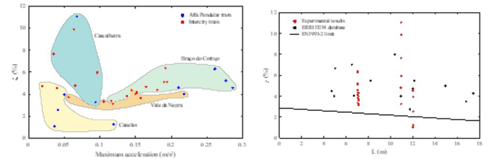
Figure 61-2 Damping coefficient estimates based on the Prony method for the four filler-beam bridges as function of the maximum acceleration (left) and the span length (right).
