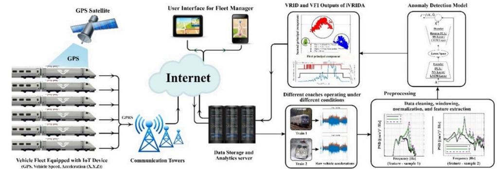
Figure 41-1 Intelligent Vehicle Running Instability Detection Algorithm (iVRIDA-fleet) Framework for X2000 fleet.
