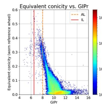
Figure 40-3 Equivalent conicity vs. GIPr
