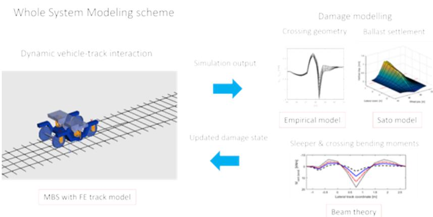
**Figure 8-1** Schematic illustration of this version of the Whole System modelling scheme. Simulation of dynamic vehicle-track interaction using multibody simulation with a finite element track model give input for damage modelling that in turn provides damage increments for crossing geometry and ballast settlement before the next iteration.
