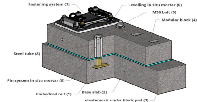
Figure 62-2 3MB fastener-block-pin assembly
