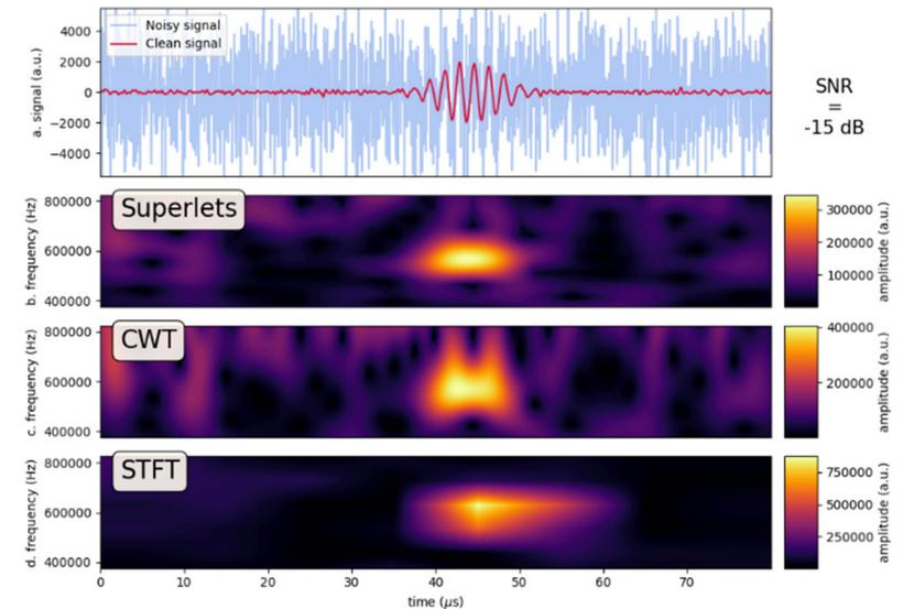
Figure 22-2 Comparison of time-frequency representations: Short Term Fourier Transform (STFT, bottom), Continuous Wavelet Transform (CWT, middle) and Superlets (top)
