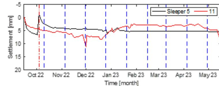
Figure 16-2 Evolution of unloaded sleeper displacement (settlement) over time for sleepers 5 and 11. Dashed vertical lines mark the accumulated traffic load, with each pair of lines representing 1 MGT
