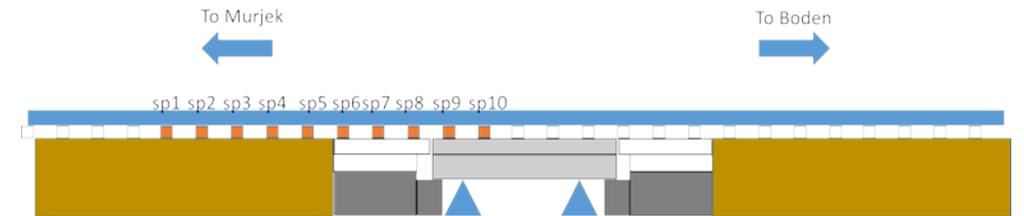
Figure 26-1 Schematic of the field measurement site
