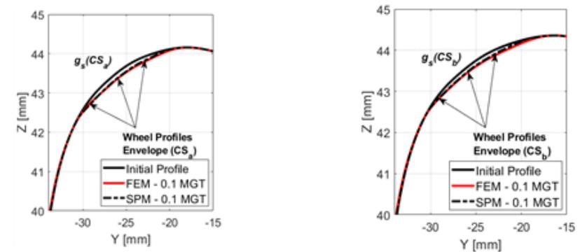
Figure 9-3 Rail profile evolution (FEM simulation results comparison with the SPP model simulation results for the two chosen cross-sections positioned along the turnout).
