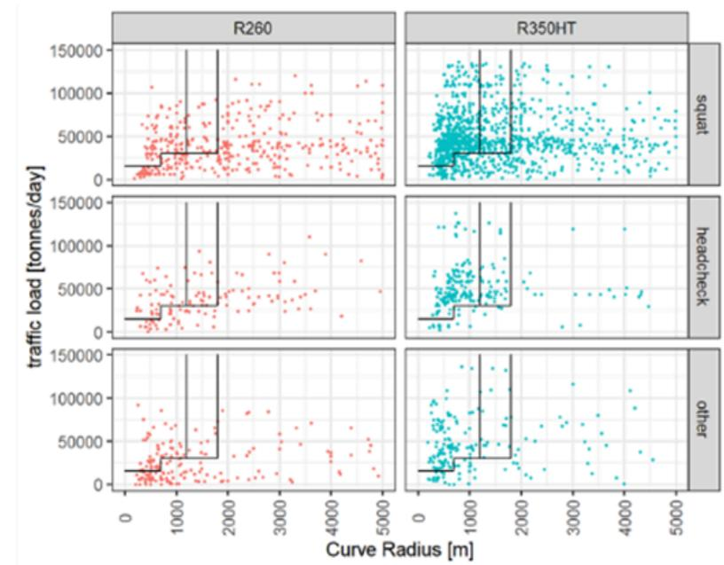
Figure 43-1 UT defects, depending on load per day and radius. The black lines correspond to the steel usage chart currently in use. N ≈ 3000
