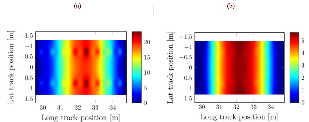
Figure 14-2 Distribution of maximum bending moment [kNm] leading to longitudinal stresses in the concrete panel: (a) dynamic vehicle load, (b) dead weight of the track superstructure. Both responses calculated for a 5.2 m washout below the centre of the panel
