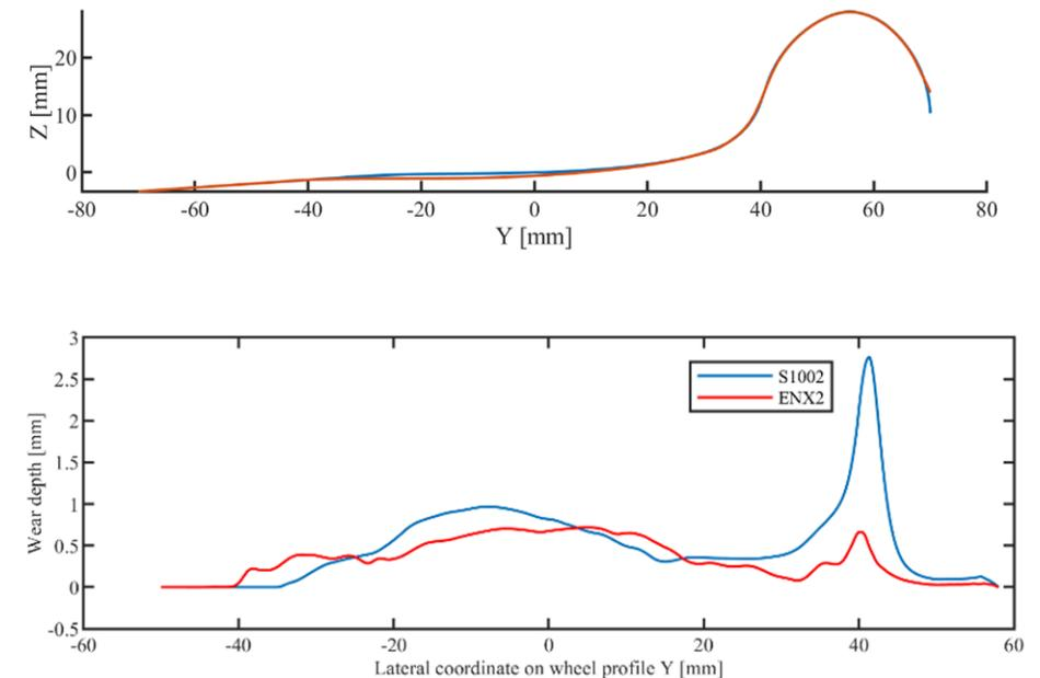
Figure 42-1 Initial wheel profiles of S1002 and ENX2 (top). Simulated wear depth of S1002 and ENX2 for outer axes after 200 000 km of running distance (bottom).
