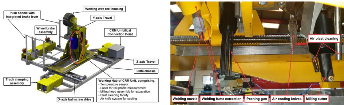
Figure 13-1 Details of the CRM machine
