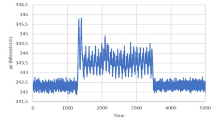
Figure 76-3 Strains during the passage of a train.
