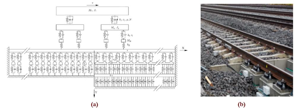
Figure 16-1 (a) Sketch of 2D vehicle and track models ( $x < 0$ : ballasted track,  $x > 0$ : slab track). (b) Overview of instrumented TZ between ballasted track and 3MB slab track at Gransjö, north of Boden in Sweden
