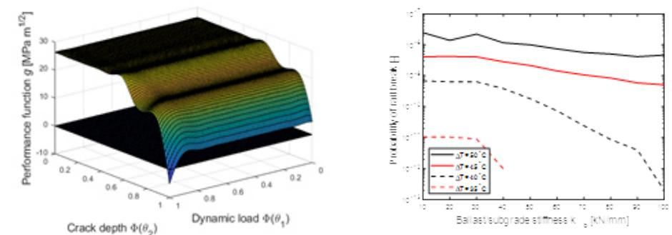
Figure 46-1 Left: Example of influence of cumulative distributions of crack depth and dynamic wheel load on performance function  $g$ . Right: Example of influences of  $\Delta T$  and  $k_b$  on probability of rail break. Freight traffic model with axle load 25 tonnes and train speed 100
