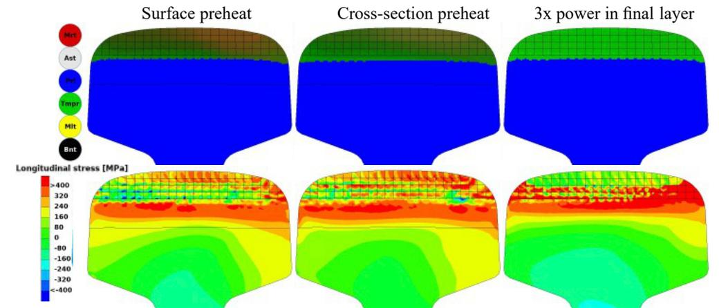
Figure 37-1 Variation of welding process parameters. Upper row: phase fractions (red: martensite, white: austenite, blue: pearlite, green: tempered martensite and/or bainite, yellow: melt and black: bainite) and lower row: longitudinal residual stress fields
