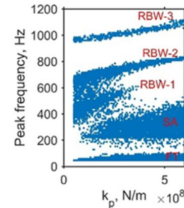
Figure 26-1 Relationships between railpad stiffness ( $k_p$ ) and peak frequencies of ABA.
