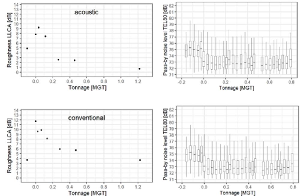
Figure 53-1 Measurements of the rail roughness single value denominator LLCA (top left and bottom left diagrams) and pass-by noise levels (top right and bottom right diagrams) of the two track sections on the southern site. The section with acoustic grinding is shown in the top row, the standard grinding process is shown in the diagrams in the bottom row. Please refer to the text for explanations.
