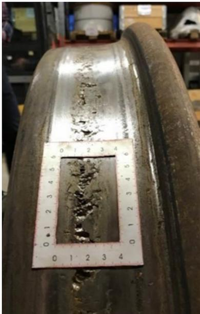
Figure 44-1 Wheel with severe rolling contact fatigue damage
