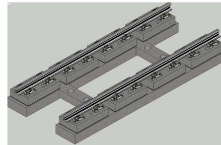
Yet ballast-less tracks brought their own problems: higher initial costs, longer installation times, increased noise and vibration, disruptive repairs in case of slab failure, and the inability to readjust geometry at settlements. The Moulded Multi Modular Block (or 3MB) system was developed to bridge the gap and address the most common slab track issues while keeping its advantages.
