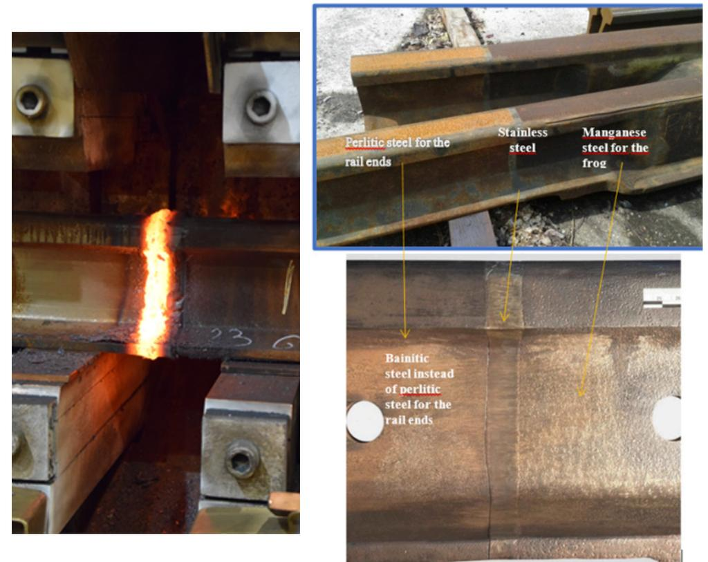
Figure 66-1 Welding, and rail ends
