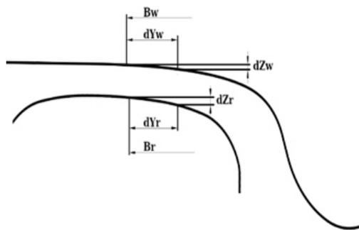
Figure 40-1 The geometrical definition of GIPw and GIPr
