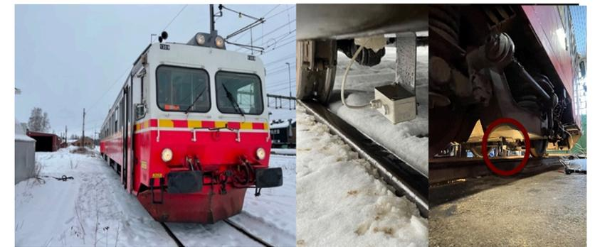
Figure 72-1 Mounting of friction level sensor on train.
