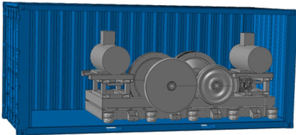
Figure 45-1 Novel full-scale brake roller test rig
