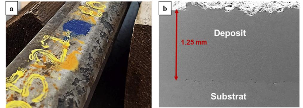
Figure 35-1 a- Physical demonstrator to be repaired, showing deep and numerous spalling defects. b- Typical repair achieved on laboratory test samples
