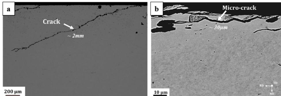
Figure 28-1 a- Typical rolling contact fatigue (here, head check) observed in R260 pearlitic steel, b- Micro-crack of less than 30µm observed in carbide-free bainite for identical sollicitation.
