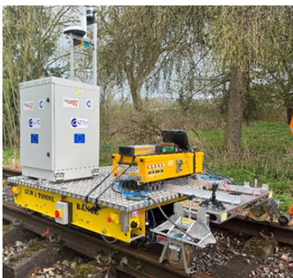
Figure 20-1 Autonomous rail inspection trolley
