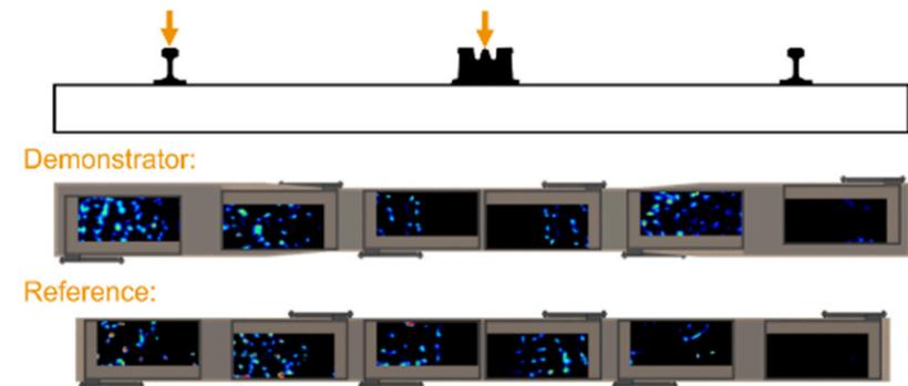
Figure 63-1 Pressure distribution under sleeper beneath frog tip
