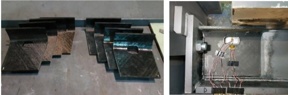
**Figure 75-2** Detail of the strengthening CFRP angles.
