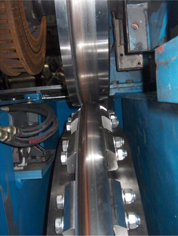
*Figure A3-8: Wheel/rail positioning at the roller rig (front view).*
