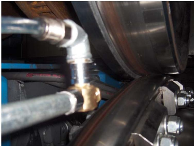
**Figure A3-7: Water-air nozzle at the roller rig**
