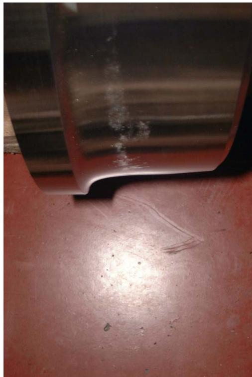
**Figure A3-2: Wheel profile with cut flange**
