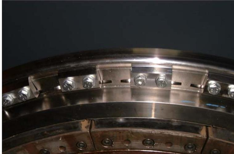
**Figure A3-3: Rail head, mounted by collets**
