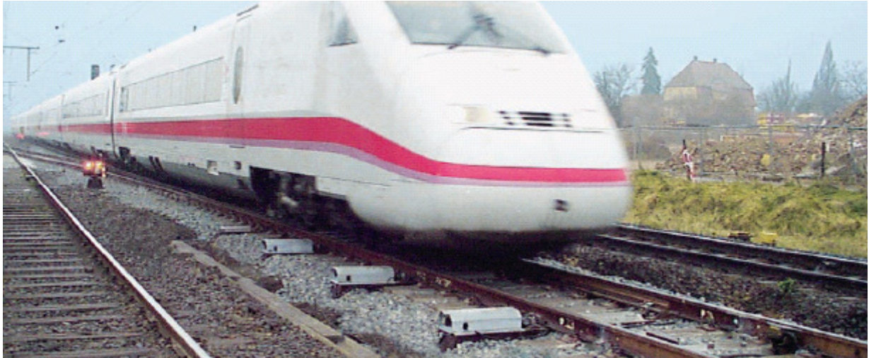
Figure 15 - A mark II ICE passes over a switch driven by 3 S700V point machines
