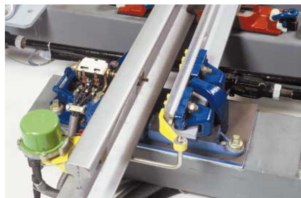
Figure 13 - (left) Vossloh Paulvé detector; (right) Vossloh VCC locking device
