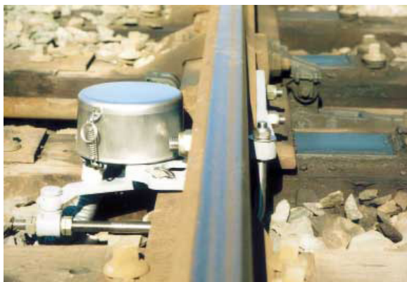
Figure 13 - (left) Vossloh Paulvé detector; (right) Vossloh VCC locking device
