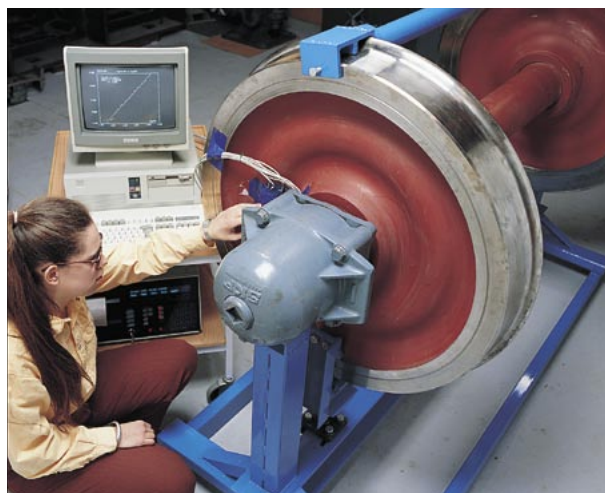
PhD student Åsa Fenander (doctorate earned in May 1997) of project TS3 inspecting an instrumented wheelset in the Chalmers Solid Mechanics laboratory. For a photo of Tore Dahlberg, see page 63
