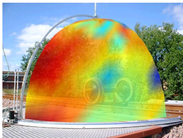
Visualization of the noise emitted from a wheel prototype as measured in the RNTR at frequency 875 Hz in project VB4. Red indicates a high level of sound pressure whereas blue indicates a low level. A reflecting ground surface is used in this experiment. Photo taken in 2002
