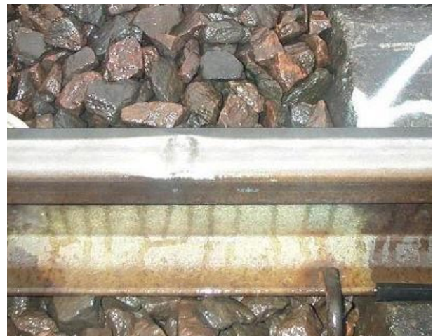
Repetitive indentation marks with spacing 3.1 m from a severely damaged wheel
