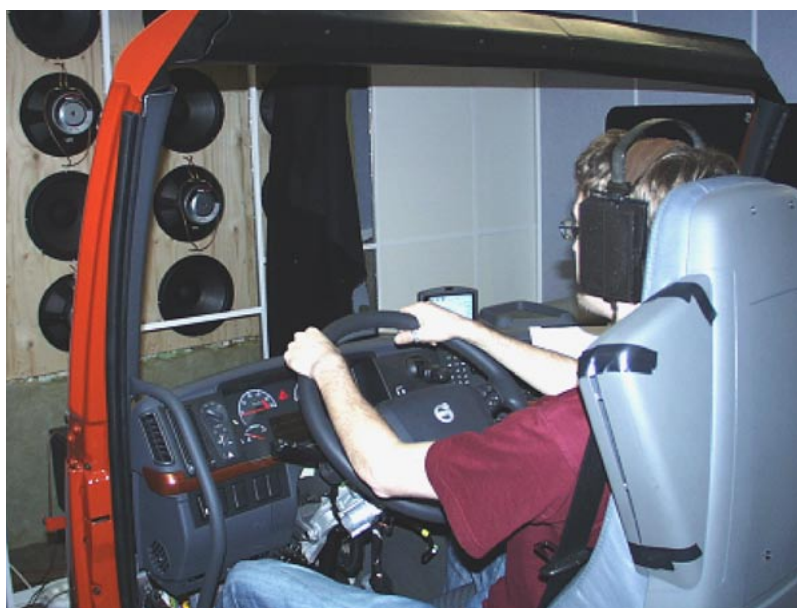
Example of an experimental set-up at Chalmers Applied Acoustics which is being used to simulate the sound and vibration properties of a transmission line in a heavy vehicle
