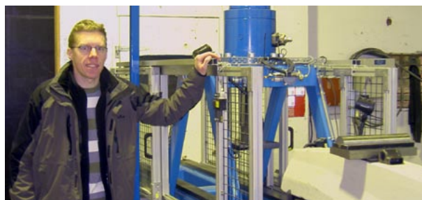
Dr Rikard Bolmsvik at Abetong Teknik's sleeper testing machine in the factory at Vislanda (Sweden)
