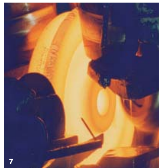
6. Reprofiled a wheelset in the Duroc maintenance shop at Notviken (Luleå) 7. Rolling of a forged Lucchini wheel
