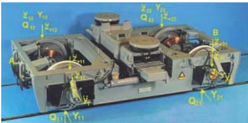
Instrumentation of non-powered X2 bogie as used during the track force measurements in October 2002 (courtesy TrainTech Engineering Sweden)
