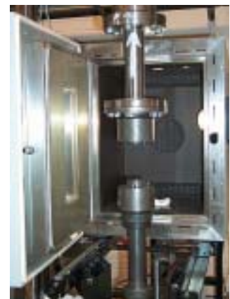
Low-temperature chamber mounted on fatigue test rig in project MU13
