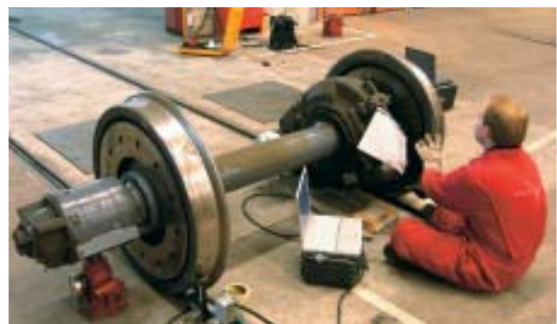
Measurement in project TS5 of wheel out-of-roundness on powered wheelset of a regional train as performed in October 2002 by the Danish consulting firm Ødegaard & Danneskiold-Samsøe A/S at Bombardier Transportation in Västerås. Three mechanical probes, 10 mm axially apart, follow the tread surface while the wheelset is slowly rotated by hand
