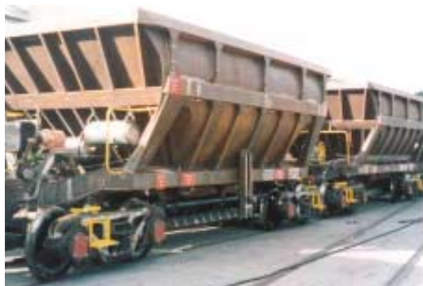
Pre-series LKAB iron ore wagon with Pneumatic Brake Unit (PBU), including brake cylinder, as delivered by Transwerk in October 2000
