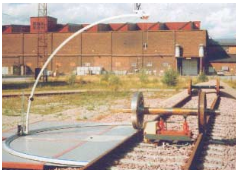
Part of test rig for noise measurements in projects VB3 and VB4. The perforated prototype wheel in project EU2 is here being investigated
