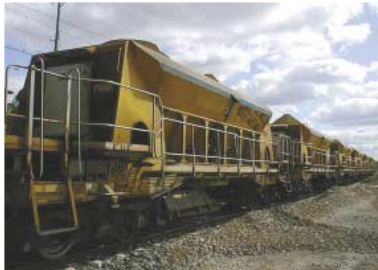
Loaded wagons with out of-round wheels at Grundbro during the test campaign in project TS5
