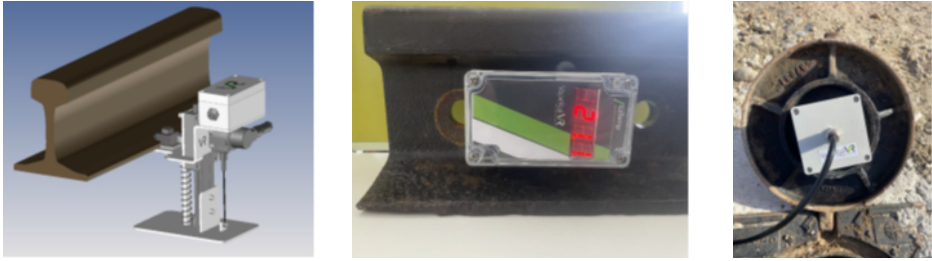
Figure 23-1 Examples of sensor node integration: (a) Acceleration sensor, (b) Temperature sensor, (c) Water level sensor
