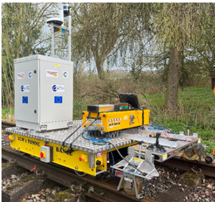
Figure 20-1 Autonomous rail inspection trolley
