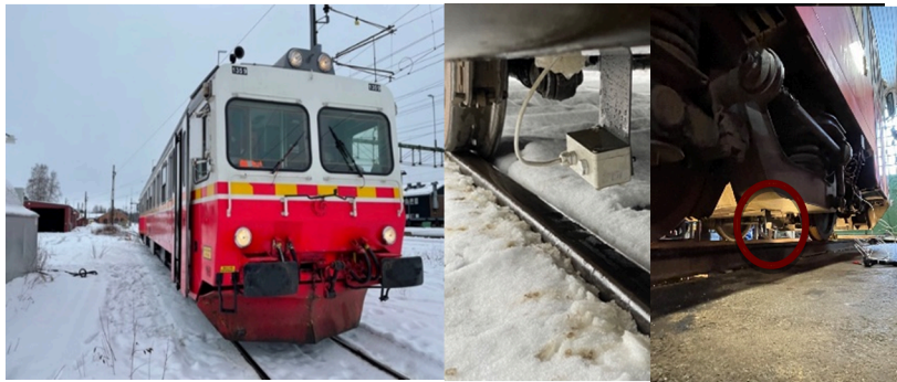
Figure 72-1 Mounting of friction level sensor on train.
