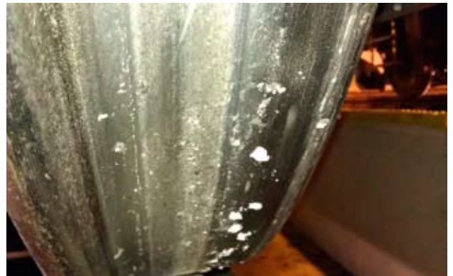
Example of damage as studied in project MU22: ice and snow trapped in initiated RCF cracks on the running surface of a wheel
