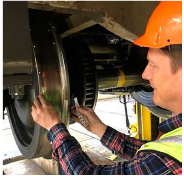
Michele Maglio scanning a wheel tread in the Luleå workshop and Tore Vernersson applying reflective points on the running surface of a wheel. Photos by Tore Vernersson and Michele Maglio
