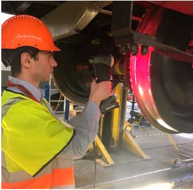
Michele Maglio scanning a wheel tread in the Luleå workshop and Tore Vernersson applying reflective points on the running surface of a wheel. Photos by Tore Vernersson and Michele Maglio
