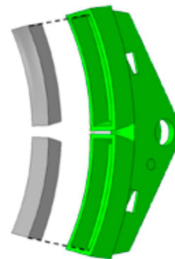
Proposed (and numerically investigated) novel type of brake block with organic composite material (here shown in gray) inserted into a shell of sinter material (green). From CHARMEC's contribution to Fr8Rail Deliverable D4.4
