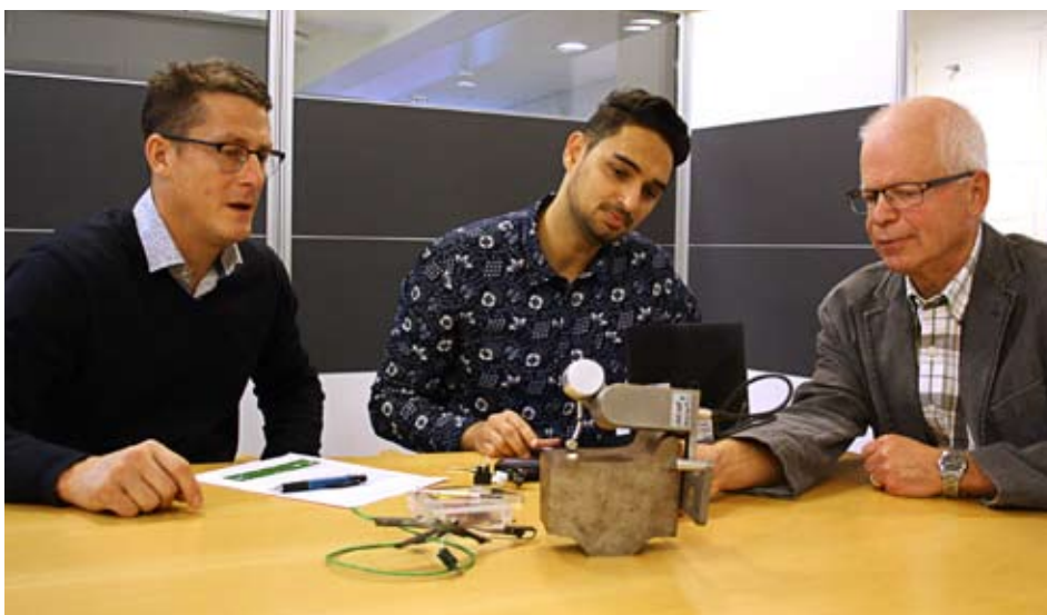
PhD student Mandeep Singh Walia in project SD10 measuring a wheel profile using the MiniProf equipment device at Roslagsbanan Depot in Stockholm in June 2018. Together with Docent Tore Vernersson (left) and Professor Roger Lundén (right)
