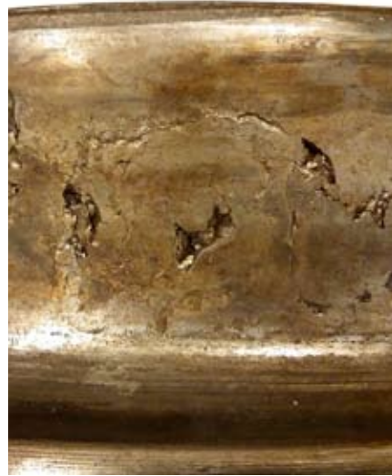
Typical rolling contact fatigue (RCF) cluster on a wheel tread. Photo by Robin Andersson
