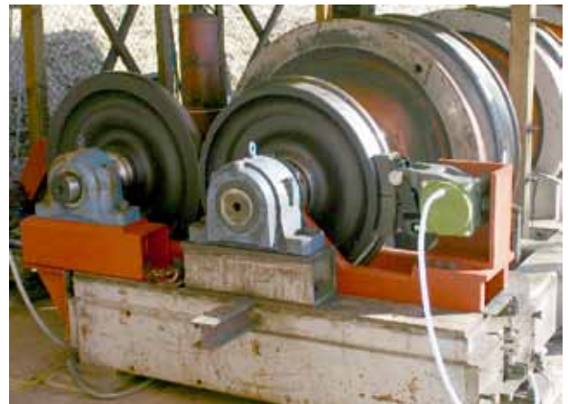
Photo of an experimental test set-up at Surahammar with a tread-braked wheel in rolling contact with a "rail-wheel". One slotted composition block (configuration 1Bg) is used, see figure on page 81
