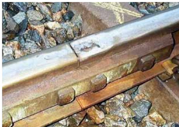
Damaged insulated joint at Järna, south of Stockholm. Running direction of train is from left to right. Measurements in project SP11 showed that the wheel of an X2 train travelling at 185 km/h flies over the cavity and then bounces twice with a peak contact force of 350 kN
