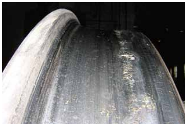
Example of observed damage on freight wheel
