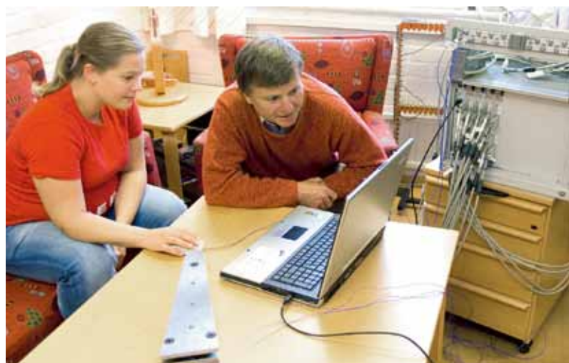
PhD student Johanna Lilja (licentiate gained in November 2006) and her supervisor Professor Thomas Abrahamsson in project TS9. On the table lies one of the 32 three-point load-measuring cells (i.e., adding up to a total 96 sensors) which were placed on the bottom surface of the test sleeper. Photo taken in 2006
