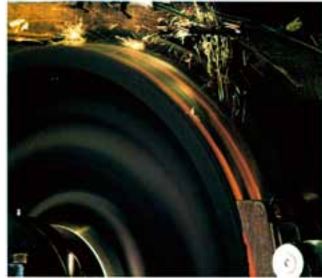
Photo of a cast-iron brake block in operation on the test rig at Surahammar in projects SD1 and EU1
