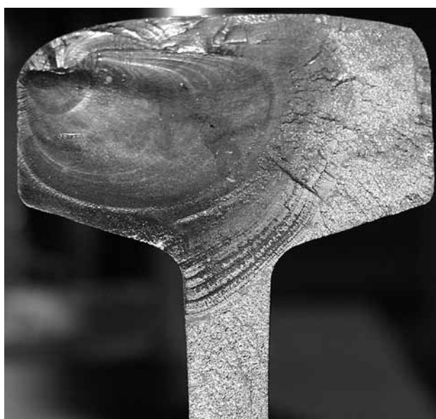
Head check crack propagating to full rail failure on Malmaban (Iron Ore Line) in Northern Sweden
