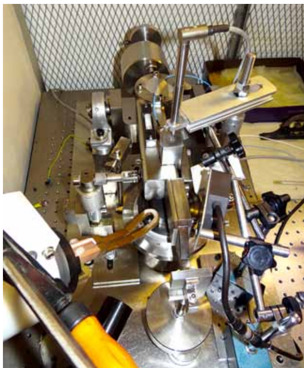
Part of equipment used in experiments at KTH. Rotating disc with pin is seen in the middle with induction heater in front of it. Detail with disc and pin above
