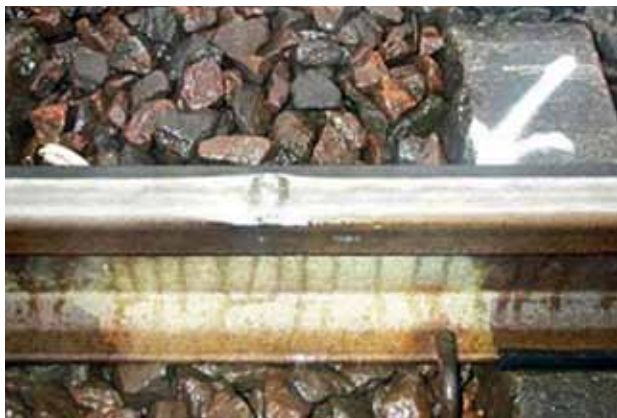
Repetitive indentation marks with spacing 3.1 m from a severely damaged wheel
