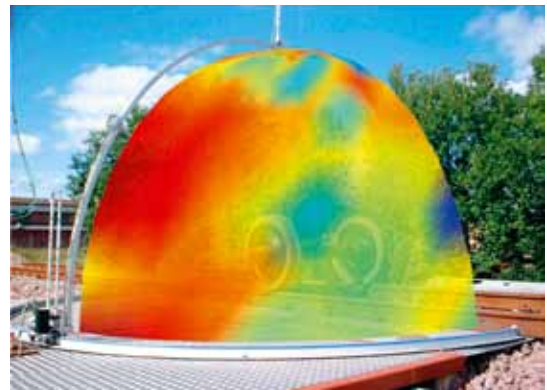
Visualization of the noise emitted from a wheel prototype as measured in the RNTR at frequency 875 Hz in project VB4. Red indicates a high level of sound pressure and blue indicates a low level. A reflecting ground surface is used in this experiment. Photo taken in 2002
