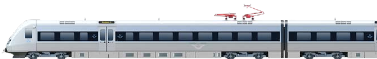
A forerunner to this SJ 3000 train holds the Swedish high-speed record of 303 km/h. This record was achieved in 2008 during a testing activity within a research project in a collaboration between Trafikverket, Bombardier, SJ, KTH, and Chalmers. Courtesy: SJ
