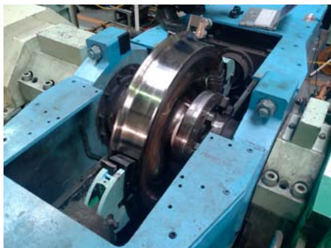
Tread brake testing at the Railway Technical Research Institute (RTRI) in Tokyo, Japan, in the collaborative experimental work between CHARMEC and RTRI, see project SD11. The test rig is equipped with a Lucchini wheel and Japanese composite brake blocks
