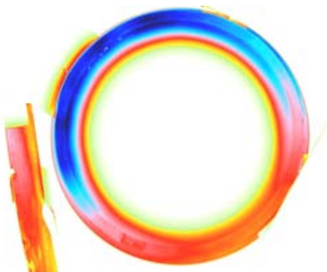
Thermographic image of a tread-braked wheel during braking. Note mirror to the left, providing view of the tread
