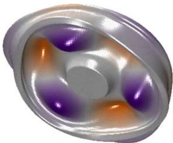
Left: Vibration pattern of a wheel in an axial mode (eigenfrequency 2120 Hz) with three nodal diameters and one nodal circle. Right: Acoustic directivity of this mode at 1000 Hz
