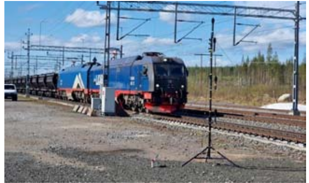
Rolling noise measurements at the demonstrator of the 3MB slab track on the Iron Ore Line in northern Sweden in May 2023
