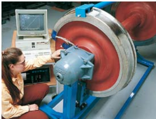
PhD student Åsa Fenander (now Åsa Sällström; doctorate earned in 1997) of project TS3 inspecting an instrumented wheelset in the Chalmers Solid Mechanics laboratory
