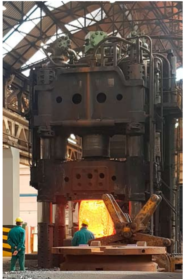
A 40-tonne ingot placed in the 4 200-tonne open-die forging press (now replaced by a new 7 000-tonne press) to obtain a special tool steel block at Lucchini RS in Italy
