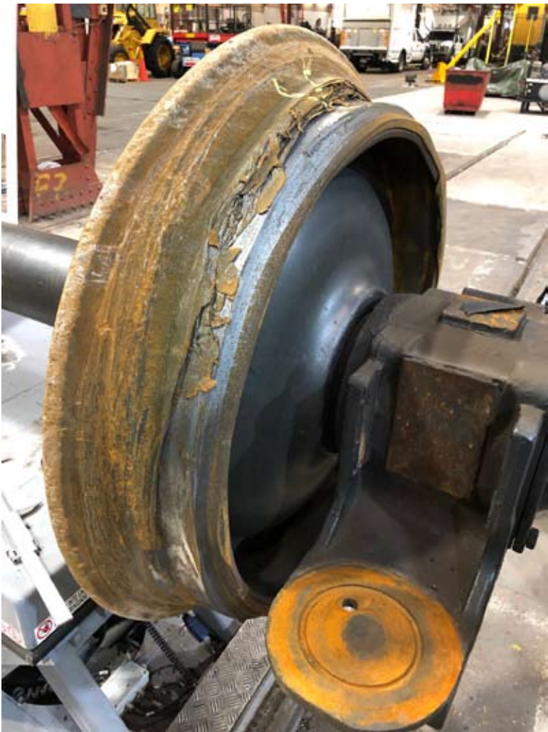
Extreme material damage of a freight wheel occurred following an event of locked tread brakes, resulting in very high temperatures and hot rolling of the wheel rim from wheel-rail contact
