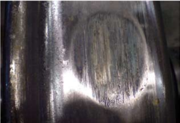
Example of a wheel impact load detector (left photo by Matthias Asplund, Trafikverket) used for identifying damaged (out-of-round) wheels (see example on the right), which may cause detrimental loading of the track, infrastructure failures, and traffic disruptions
