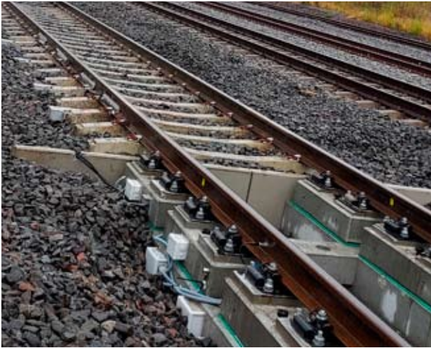
Overview of test site at Gransjö involving a transition zone between a ballasted track and a 3MB slab track. Instrumented sleeper with an accelerometer and a displacement transducer
