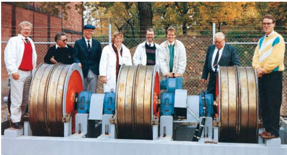
The brake test rig (inertia dynamometer) at Surahammar (used in projects SD1, SD4, EU1 and EU8) at its inauguration in 1989. From the left: Roger Lundén, Josef Rauch (from Sura Traction, now Lucchini Sweden), Bengt Åkesson, Elisabet Lundqvist and Lennart Nordhall (both from Sura Traction), Mikael Fermér (from Chalmers Solid Mechanics), and Nils Månsson and Sven A Eriksson (both from SJ Machine Division)
