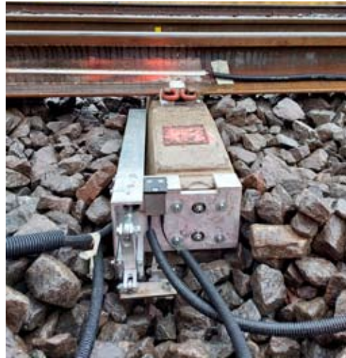
Overview of test site at Gransjö involving a transition zone between a ballasted track and a 3MB slab track. Instrumented sleeper with an accelerometer and a displacement transducer
